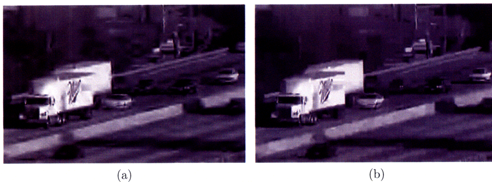
Figure 5-23: Beertruck (cropped 531 \times 341 ) I-frame: (a) JPEG2000 (PSNR = 27.9 dB); and, (b) H.264 (PSNR = 27.9 dB).
