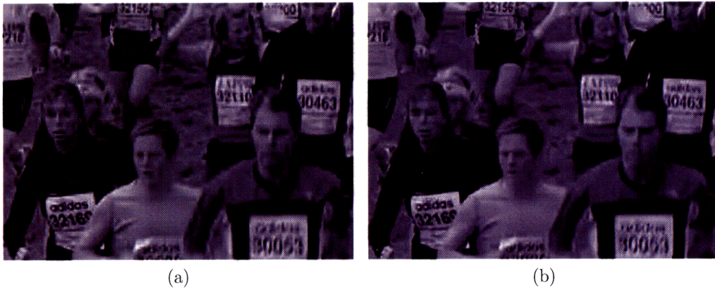
Figure 5-12: CrowdRun (cropped, 321 \times 231 ): (a) JPEG2000 (PSNR = 28.1 dB); and, (b) H.264 (PSNR = 28.1 dB).
