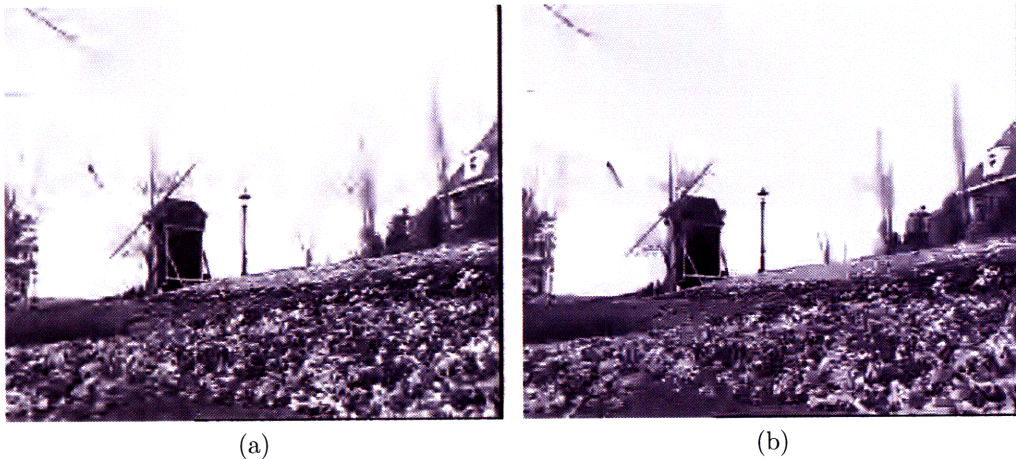
Figure 5-20: Flower (CIF) I-frame: (a) JPEG2000 (PSNR = 22.8 dB); and, (b) H.264 (PSNR = 22.8 dB).
