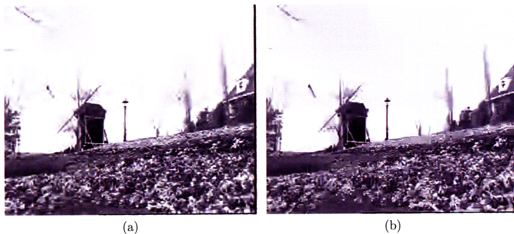
Figure 5-21: Flower (CIF) first P-frame: (a) JPEG2000 (QPPSlice = 44, PSNR = 22.9 dB); and, (b) H.264 (QPPSlice = 44, PSNR = 22.9 dB).
