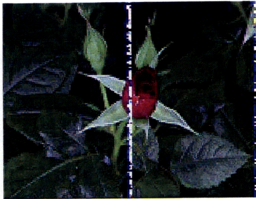
Figure 4-10: Received Image with Payload Length of 123 bytes and nSampSlot of 5
