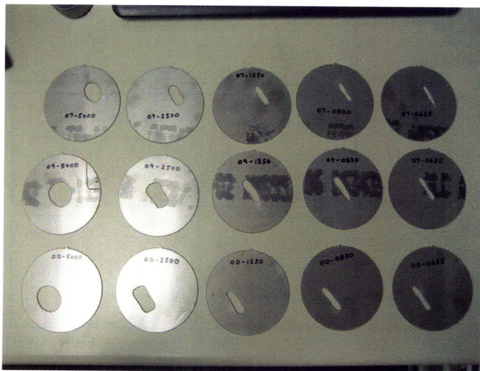
Figure B-6: Aperture plates fabricated based on the images shown in Fig B-5 (b) and used to mimic the L1 aperture shown in Fig B-5 (a) during the FY2007 campaign.
