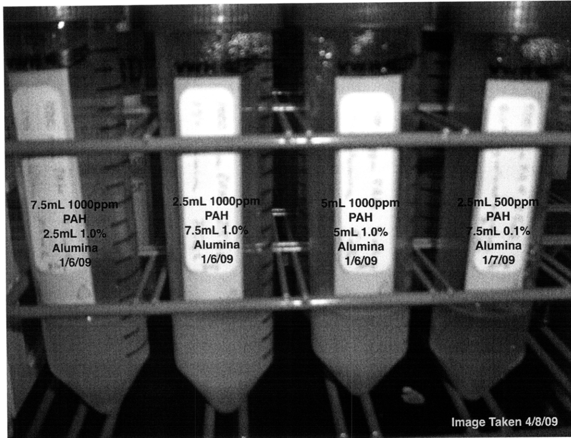
Figure 34: Alumina and PAH mixtures 3 months after initial preparation. As can be seen, no agglomeration, settling, or discoloration has occurred in these samples.
