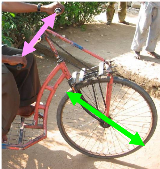
Inefficient gear ratios
