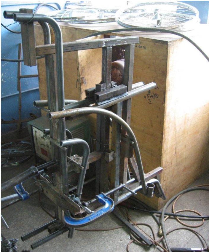
Current Whirlwind jig with separate left and right sides
