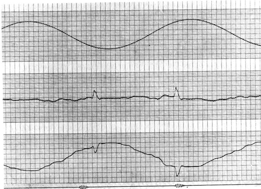
Fig. XVIII-4. Experiment results of dynamic process identification of the postural control system. Upper, input; lower, tracking signal on which is superimposed the impulse response; middle, difference of the two. The paper is running at 100 mm/sec; vibration of the needle is clearly shown at this speed.
