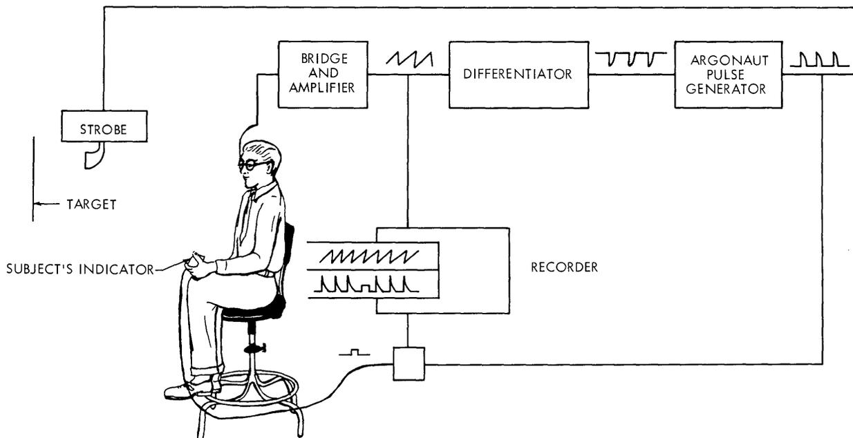
Fig. XVIII-2. Schematic representation of experimental apparatus.
