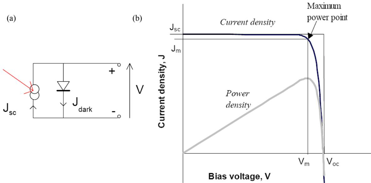
**Figure 2.2** (a) Equivalent circuit of an ideal solar cell, and (b) current-voltage (black) and power-density (grey) characteristics of an ideal cell.<sup>[17]</sup> If the fill factor  $FF = 1$ , the current-voltage curve would follow the outer rectangle.
