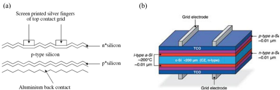
**Figure 2.3** (a) Schematic cross-sectional view of a silicon solar cell with screen printed contacts.<sup>[18]</sup> (b) Illustration of a Sanyo high-efficiency Si heterojunction with intrinsic thin layer (HIT) solar cell that has an efficiency of up to 22.3%.<sup>[5]</sup>
