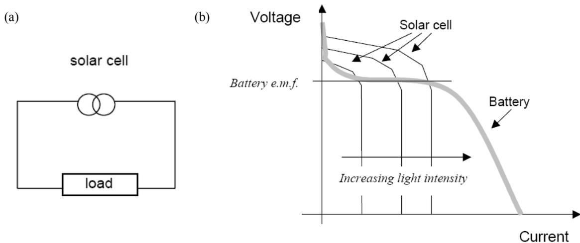
**Figure 2.1** (a) Schematic diagram of a solar cell replacing a battery in a simple circuit, and (b) voltage-current curves of a conventional battery (grey) and a solar cell under different levels of illumination.<sup>[17]</sup> A photovoltaic cell is essentially a current source that delivers a constant current for any given illumination level while the voltage is determined largely by the resistance of the load.
