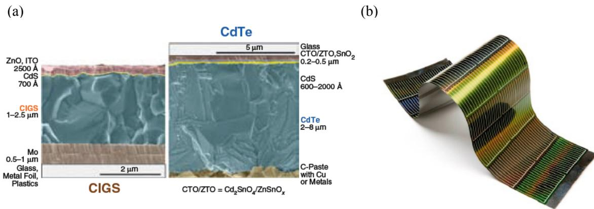
**Figure 2.4** (a) Cross-sectional SEM micrographs of a CIGS solar cell (left) and a CdTe cell (right).<sup>[5]</sup> (b) Global Solar CIGS Flexible Solar Cells.<sup>[28]</sup>
