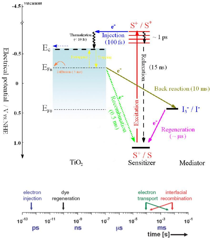
**Figure 3.2** State diagram representation of the reaction kinetics in the DSC (top) and the corresponding timescale (bottom).<sup>[6]</sup> Forward processes consist of (1) light absorption, (2) electron injection, (3) dye regeneration and (4) charge transport. The competing loss pathways are the (5) excited-state decay to ground and electron recombination with (6) dye cations and (7) oxidized redox couple.
