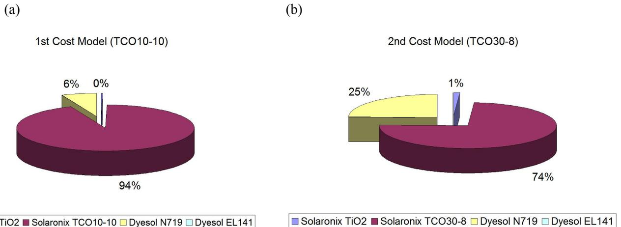
**Figure 5.2** Material cost assessment using (a) TCO10-10 and (b) TCO30-8 substrates while maintaining all other parameters constant.
