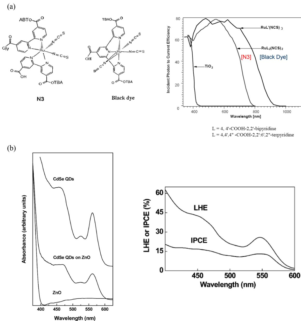
**Figure 3.5** (a) Chemical representation<sup>[48]</sup> and spectral response curve of the photocurrent<sup>[49]</sup> for the DSC sensitized by N3 and the black dye. (b) Room-temperature optical absorption spectra of a dispersion of 3 nm MPA-capped CdSe QDs in methanol and a 2 $\mu\text{m}$  long ZnO nanowire-coated FTO substrate before and after adsorption with the same QDs, and IPCE and LHE values.<sup>[55]</sup>
