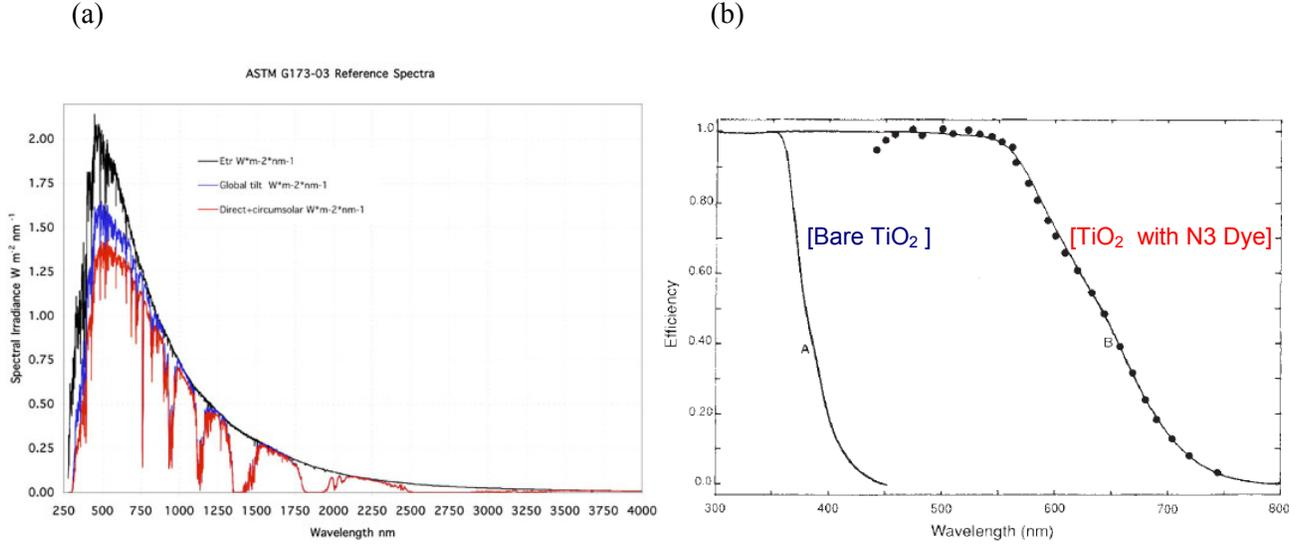
**Figure 3.3** (a) AM1.5 solar spectral irradiance.<sup>[38]</sup> (b) Absorption and photocurrent action spectra of bare TiO<sub>2</sub> film and the same film coated with a monolayer of RuL<sub>2</sub>(μ-(CN)Ru(CN)L<sub>2</sub>)<sub>2</sub> dye sensitizer supported on conducting glass.<sup>[35]</sup>
