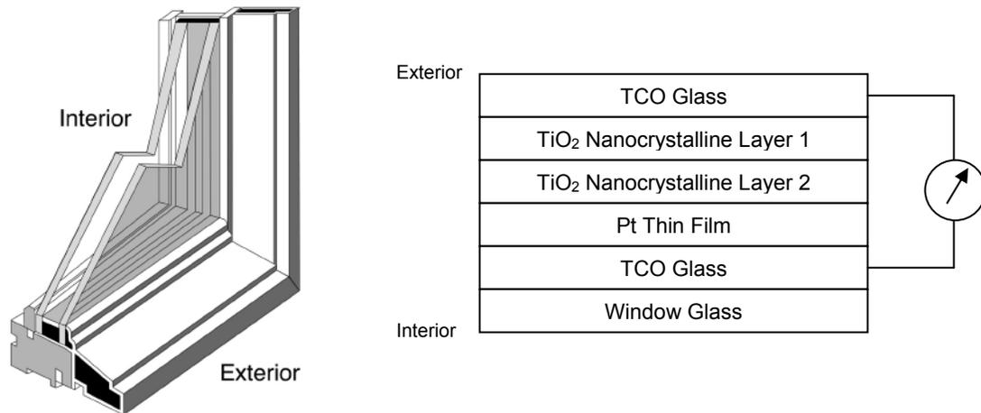
**Figure 5.1** Schematic illustration of BIPV window.<sup>[83]</sup>
