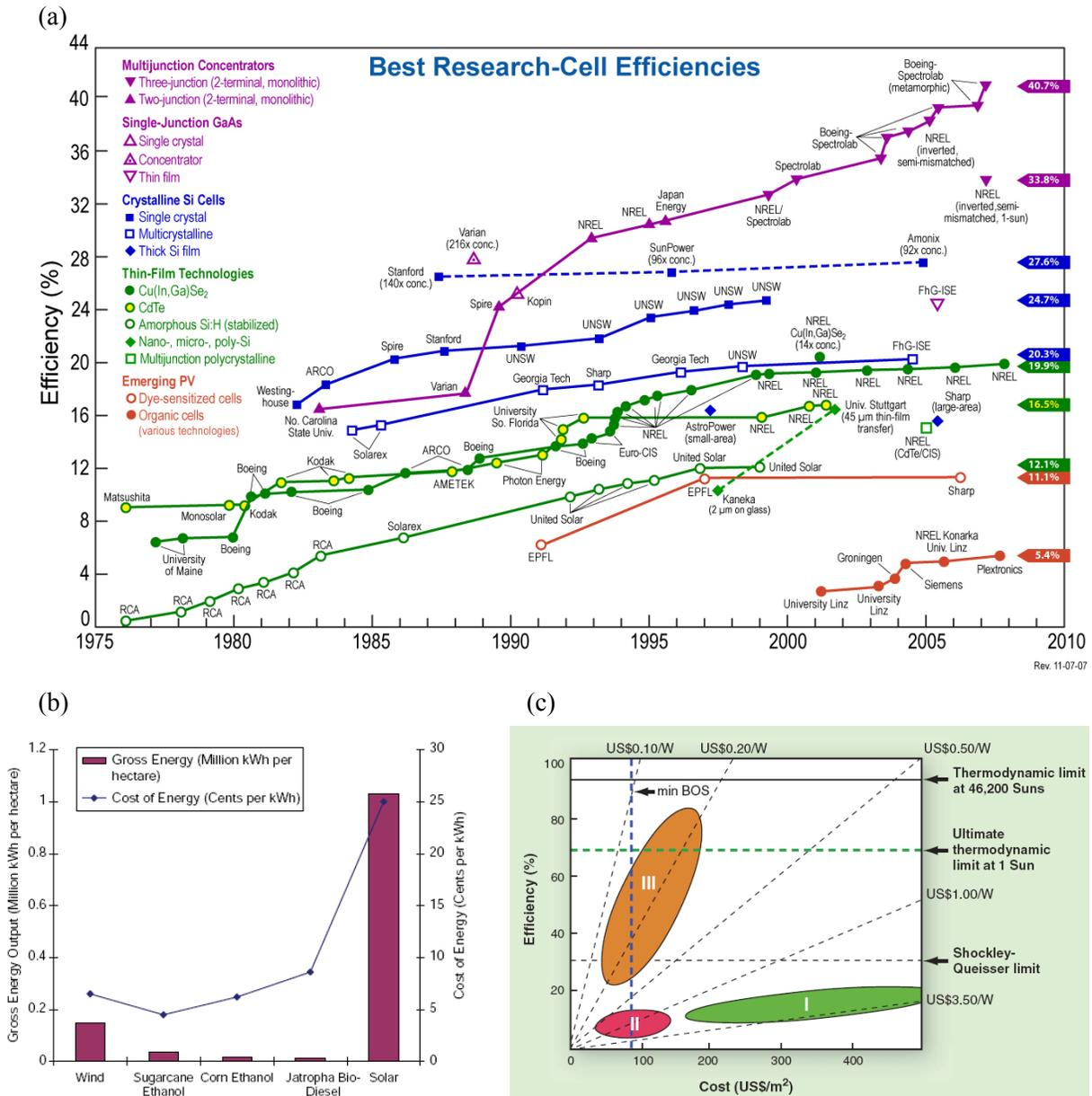
**Figure 1.1** (a) Progress of research-scale photovoltaic device efficiencies under AM1.5 stimulated solar illumination, (b) Gross energy output (million kWh per hectare) and cost (cents per kWh) of resource produced from 1 hectare of land for several renewable sources of energy, and (c) cost-efficiency analysis for I, II, and III generation of PV technologies.<sup>[5]</sup>
