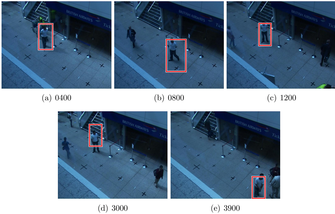
Figure 6-6: S01 Key Frames : This clip contains a single loiterer. We show our tracker’s estimate of the loiterer in several manually-selected key frames as a red bounding box. The subfigure labels indicate the frame number, for those wishing to compare and/or replicate our results.
