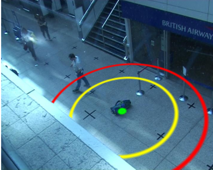
Figure 6-1: Actor Entering the Abandoned-luggage Warning Zone : In this image (frame 1120, camera 3, clip S08 ), we mark the location of a dropped piece of luggage with a green dot. The owner has just left the 2m -radius area about the bag defining a warning zone indicated by the yellow circle. After remaining outside the red circle ( 3m ) for more than 15 seconds, an abandoned luggage alarm should be generated.
