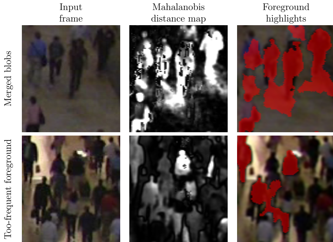
Figure 3-3: Typical Background Subtraction Failures : These image chips were extracted from background subtraction results for the frame in Fig. 3-2. In the top row, we see that the blobs from the three people in the top left get merged. The leftmost person with a blue shirt has an extra blob that includes his feet, his shadow, and the head of the woman below him with a pink blouse. The bottom row was extracted from the passageway near the top right of Fig. 3-2. In addition to merged blobs, most people are missed because pedestrians are so frequent in that area that no good background model is learned.
