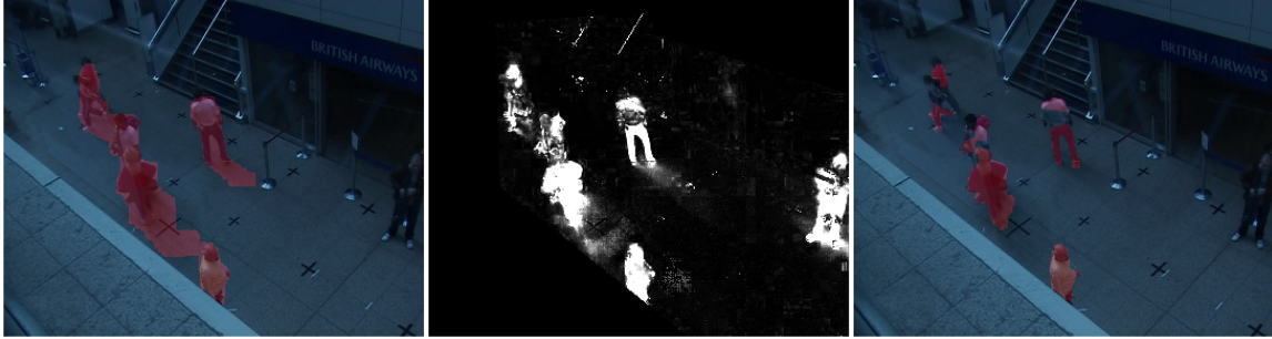
Figure 6-5: An Extreme FG/BG Segmentation Example : Here we show segmentation results for the foreground- (left) and background-biased (right) MRFs for frame 500 of clip S08 . The frame shown here is a somewhat extreme example of the different solutions found by the two MRFs. Both MRFs use the Mahalanobis distance values visualized in the middle image as the background label potential. For display purposes, the intensity is saturated at a distance of 64, twice the foreground potential for the background-biased MRF (so a 50% gray pixel sits on the classification threshold, absent any neighborhood effects).
