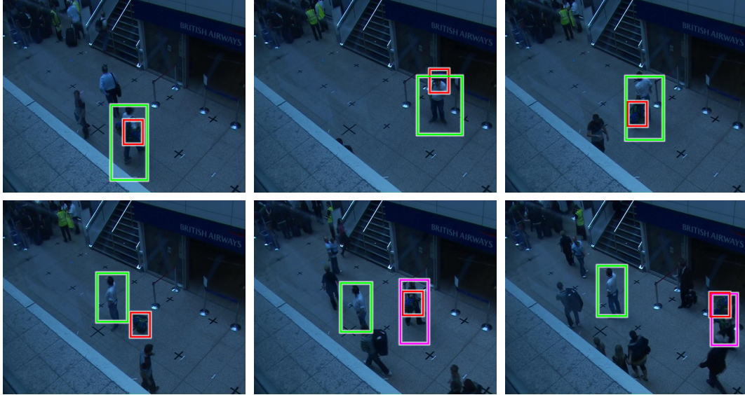
Figure 1-4: PETS 2007 Event Detection Result : Here we show tracker bounding boxes for several key frames from our event detection work for PETS 2007 [23]. The original owner’s track is visualized with a green bounding box. He sets his bag (red) on the floor, which is stolen by a thief (magenta). Full details are in §6.
