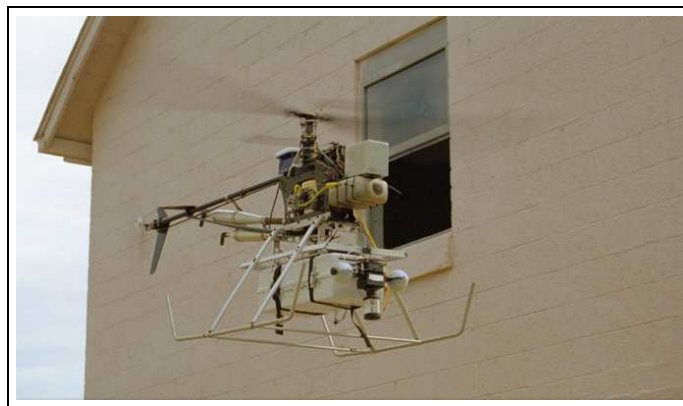
Figure 1-6: The USC AVATAR helicopter, built around a Bergen Industrial Twin RC helicopter, which is a common helicopter platform for outdoor experiments. [Photo credit: Dr. Stefan Hrabar and the USC Robotic Embedded Systems Laboratory ( http://robotics.usc.edu/resl )]
