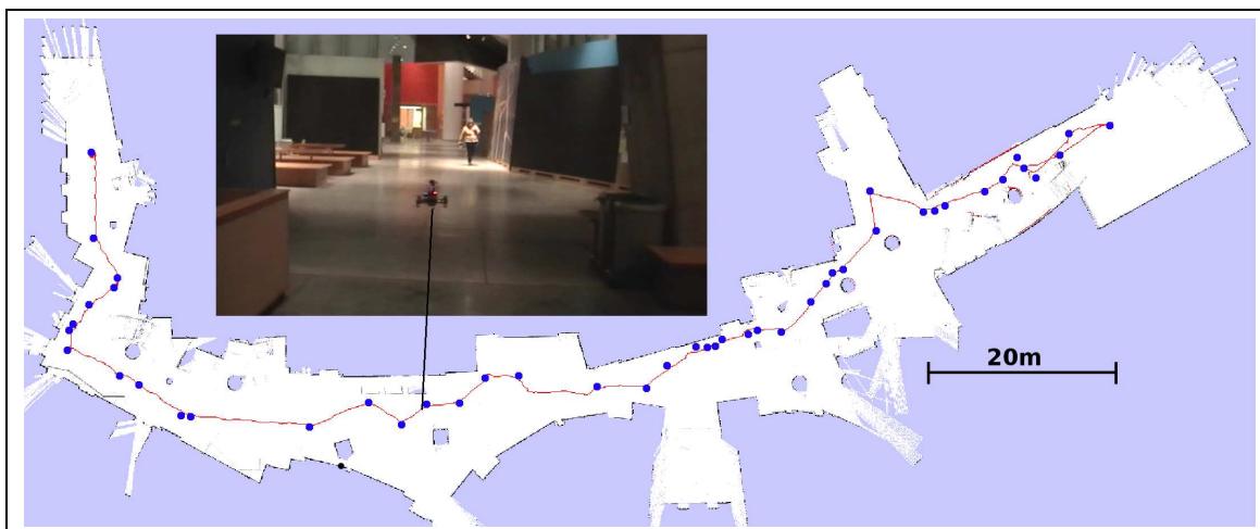
Figure 4-5: Map of the first floor of MIT’s Stata center constructed by the vehicle during autonomous flight. The blue dots indicate goal points selected by the user.
