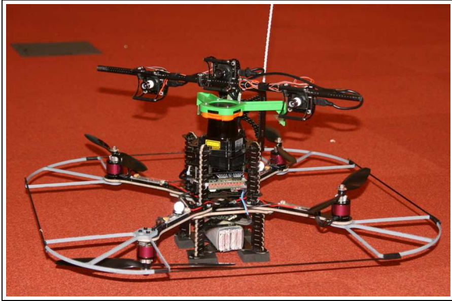
Figure 4-4: The Asctec Pelican, outfitted with both the laser range-finder and stereo camera. A third color camera is mounted in the center.
