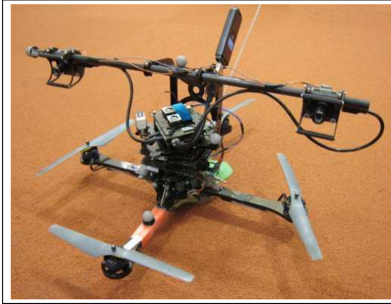
Figure 4-2: Our quadrotor helicopter equipped with a stereo camera rig, Intel Atom ® based onboard computer and USB Wifi dongle.
