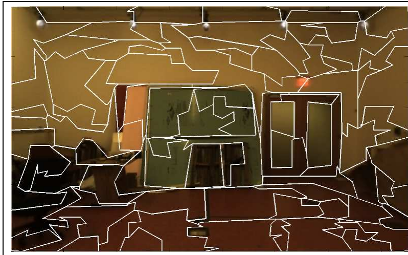
Figure 5-4: The Segmented image after applying the simplification routines.
