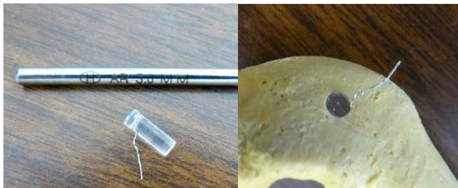
Figure 8.3 – Photograph of PMMA rods used to simulate foreign implant object. (Left) custom-made PMMA rod with threaded wire and matching 3 mm drill bit, and (right) insertion into a model 3 mm x 10 mm defect demonstrating good fit.
