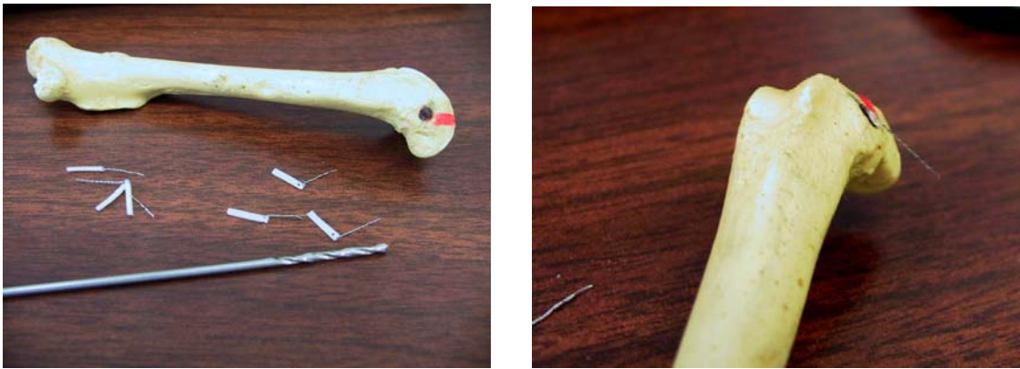
Figure 8.1 - Model femur bone showing: (left) defect site at the medial femoral condyle, along with wired bone cement rods and 8mm drill bit, (right) bone cement rod placed into the model defect to check fit.
