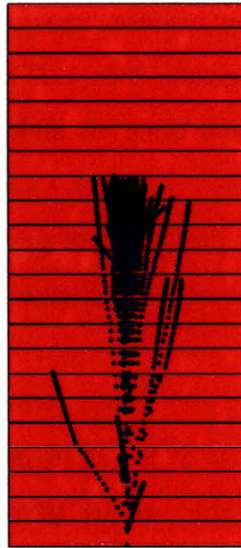
Figure 2-1: MCNPX simulation of a 150 MeV proton beam entering and stopping in a Lucite phantom. Beam enters at bottom of figure and traverses 15cm of Lucite before stopping. Note the beam broadening as the protons traverse the phantom and the distinct range of the beam. Each blue dot represents one collision between a proton and the phantom material – as the proton beam traverses more material and loses more energy, the density of collisions per unit length increases, demonstrating the higher linear energy transfer (LET) of proton beams at the Bragg peak.
