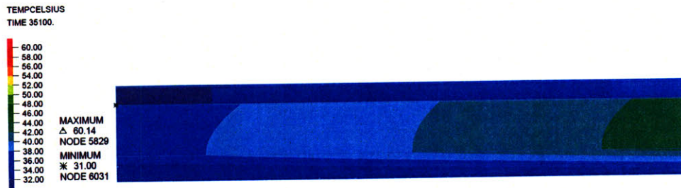
Figure 3-1: A temperature profile band plot at a time of 35100 seconds in the simulation. The entrance temperature can clearly be seen as remaining constant. The difference between the thermal properties of the materials can also be observed. Note the abrupt change between the phase-change material and the insulation. Changes in the insulation's temperature take much more time and energy than in the PCM because it has a small thermal conductivity.
