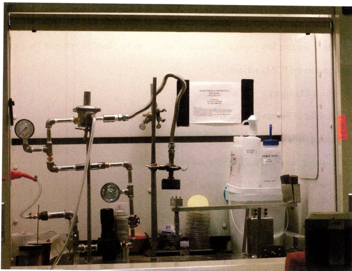
Fig. 5 The completed flame plasma treatment system in a fume hood.
