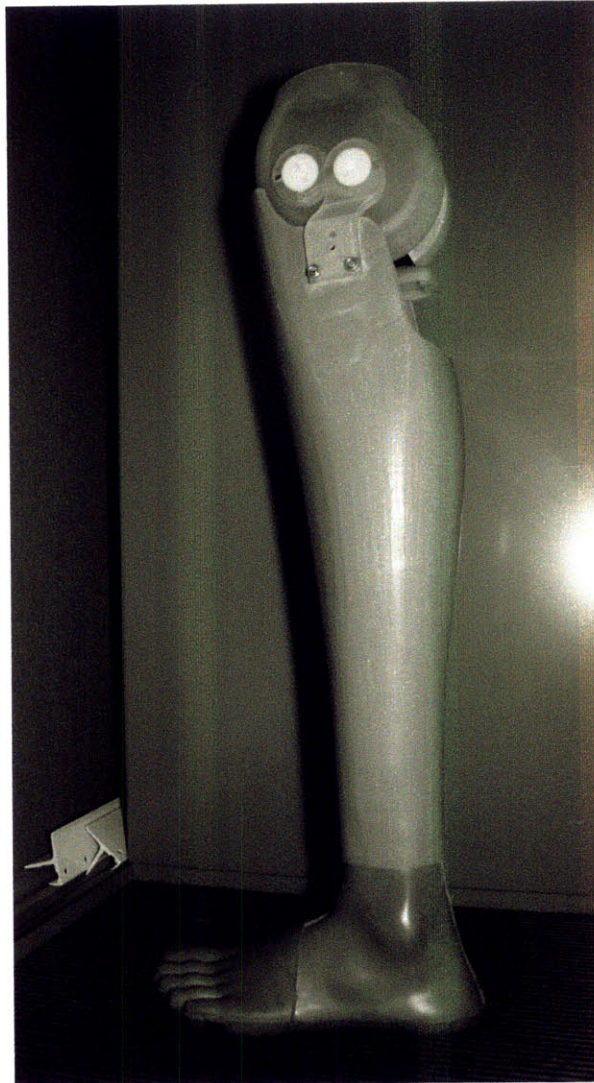
Figure 8 Exo-Knee Version 2: Final prototype of the knee before class presentations in May 2008. The prototype is functionally similar to the current design, but lacks structural stability or components designed for manufacture.
