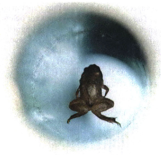
Figure 10. A frog levitated by a superconducting magnet. Photo, with a link to associated video, can be found at the Wikipedia article on magnetic levitation . The frog is unharmed by this experience.
