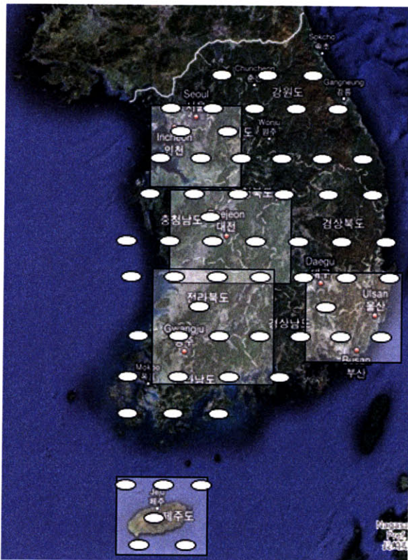
Figure 5.9: Configuration of the Navigation System Covering the South Korean Peninsula; Source: Adapted from Myoung et al, "A System Design of Stratospheric Airships for the Navigation in Korea," August 2001
