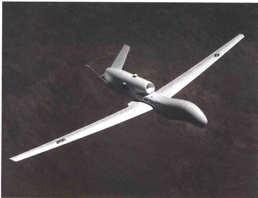
Figure 1.2: Air Force RQ-4 Global Hawk UAV; Image Source: http://en.wikipedia.org/wiki/Global_Hawk
