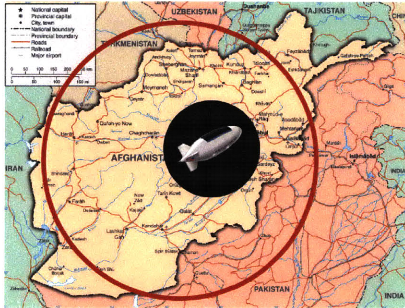
Figure 2.11: Example HALE Footprint Coverage (647 mile diameter from 70,000 feet); Source: Rand Study, "High Altitude Airships for the Future Force Army"
