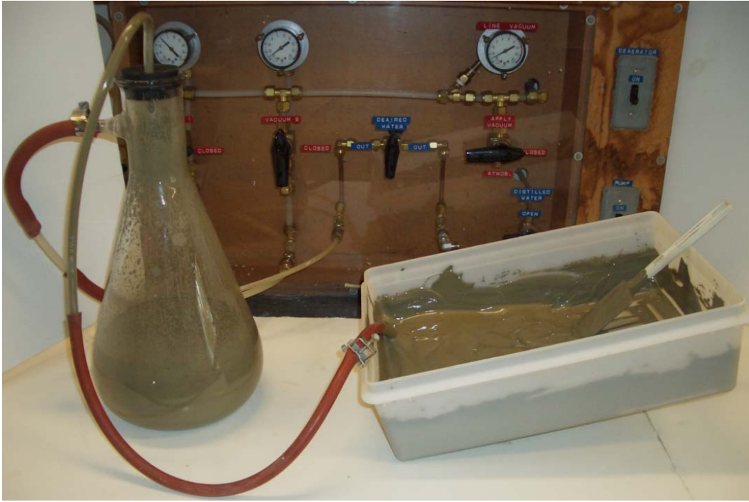
Figure 3-5: Vacuum setup used to de-air the RBBC slurry
