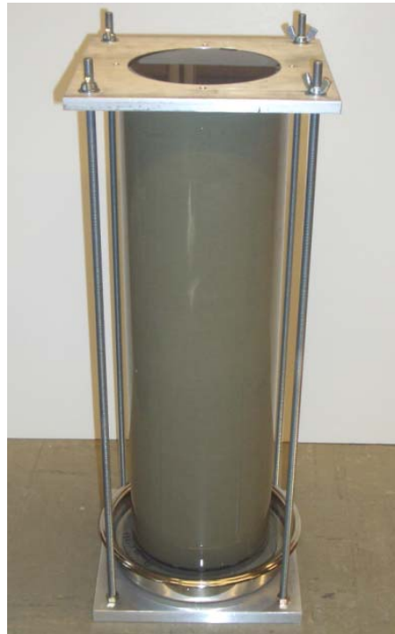
Figure 3-4: Large TWC consolidometer setup: a) schematic, b) photograph
