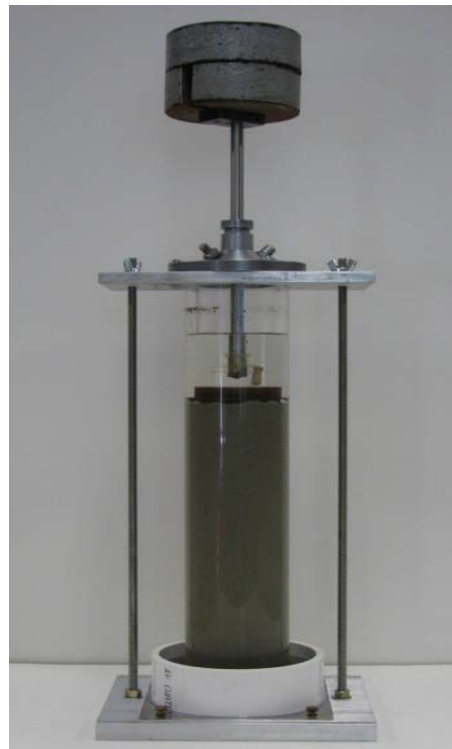
Figure 3-3: Small TWC consolidometer setup: a) schematic, b) photograph
