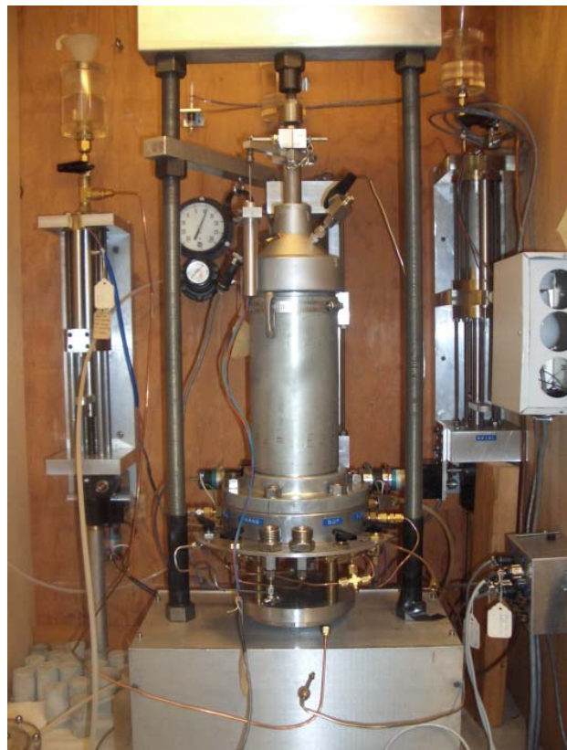
Figure 4-7: Photograph of the high pressure triaxial system inside the environmental enclosure
