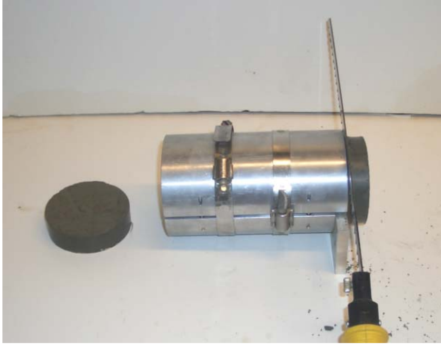
Figure 4-27: Cutting the ends of the small diameter TWC specimen using a tree saw
