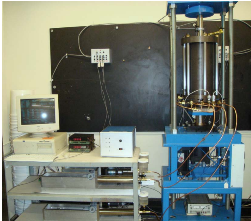
Figure 4-16: Photograph of the large diameter TWC system
