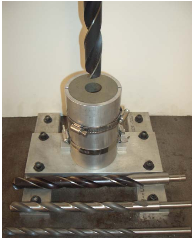
Figure 4-28: Coring of cavity for small diameter TWC specimen using drill press
