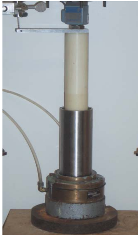
Figure 3-2: Triaxial consolidometer setup: a) schematic, b) photograph
