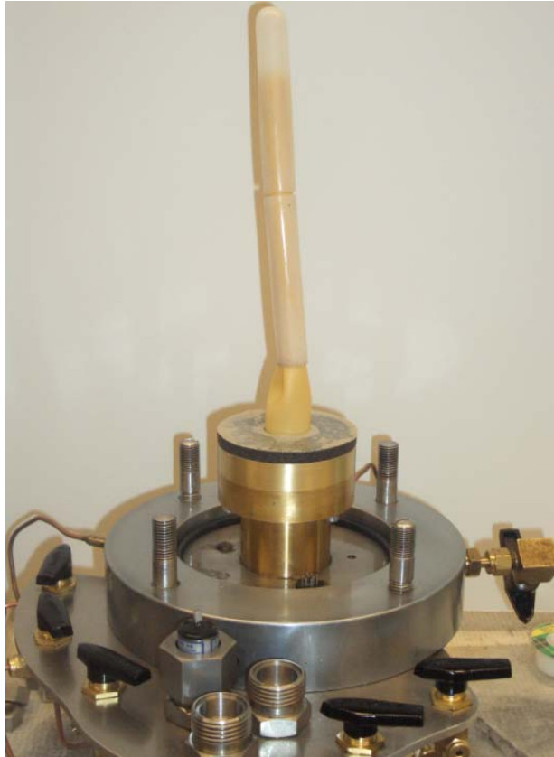
Figure 4-29: Collapsing of internal membrane using plastic tube in the small diameter TWC apparatus
