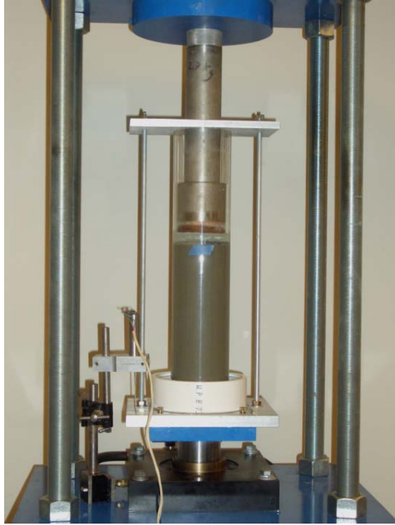
Figure 3-7: Consolidation of RBBC soil in small TWC consolidometer using high capacity load frame
