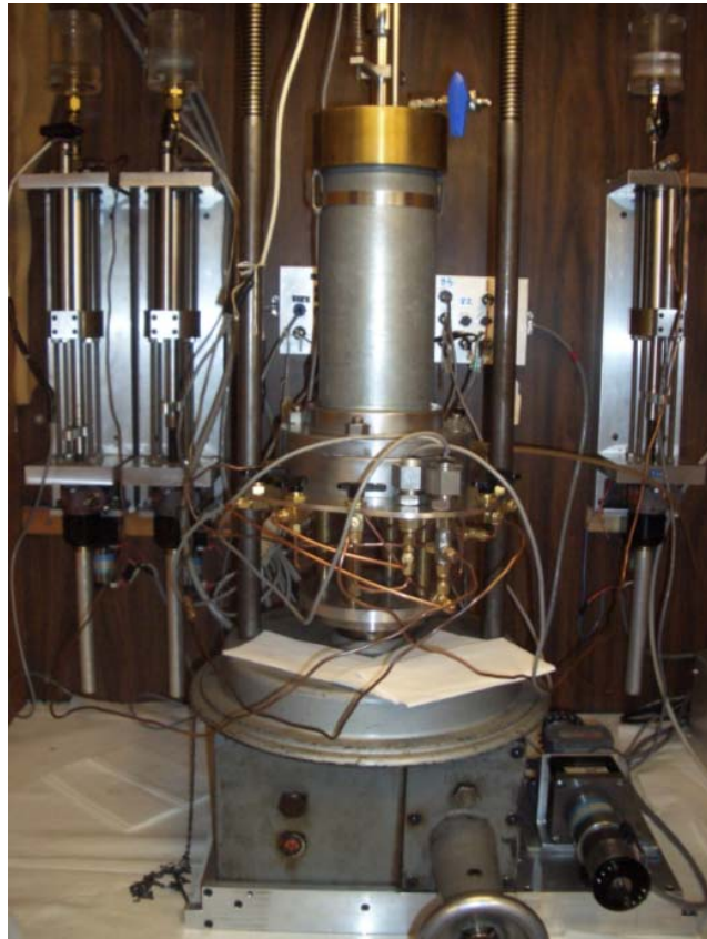
Figure 4-12: Photograph of the small diameter TWC system inside the environmental enclosure
