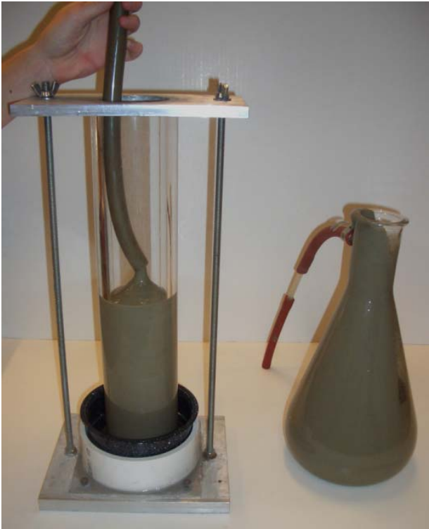
Figure 3-6: Pouring of RBBC slurry into small TWC consolidometer
