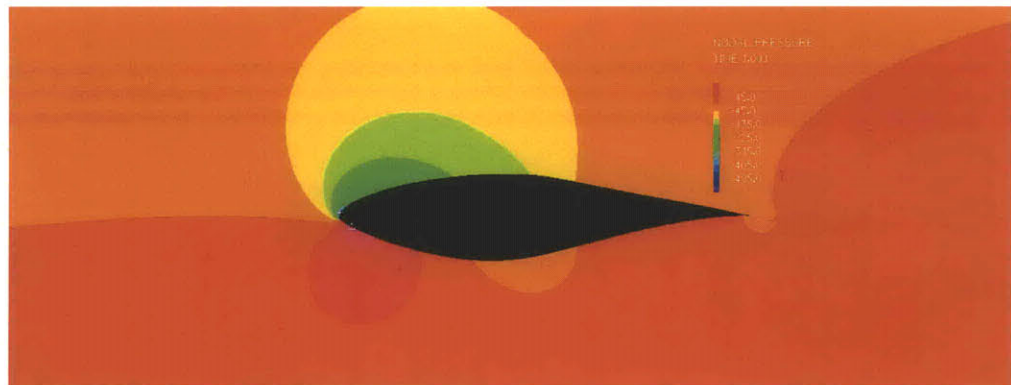
Fig. 21: S809 pressure field at RE=10E6, AoA=14°
