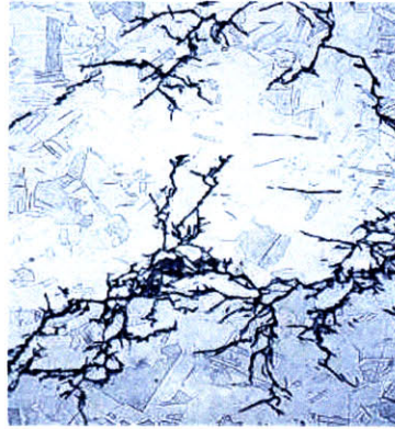
Figure 2.2 - Transgranular SCC in 316 austenitic stainless steel [12].
