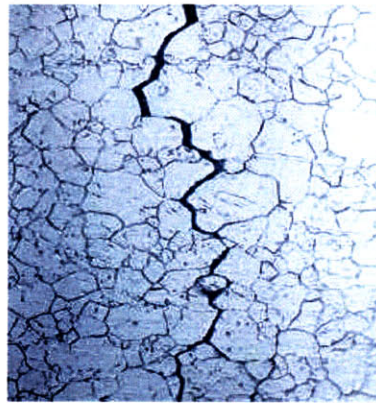
Figure 2.2 - Transgranular SCC in 316 austenitic stainless steel [12].
