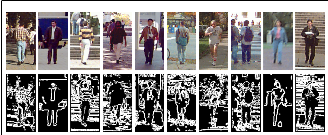
Figure 2-6: The top row shows examples of images of people in the training database. The bottom row show edge detection of the pedestrians. Edge information does not characterize the pedestrian class well.
