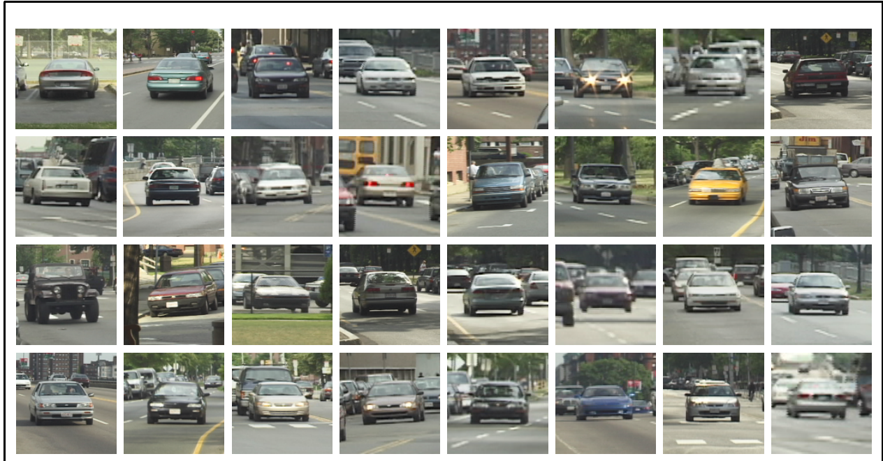
Figure 2-4: Examples from the database of cars used for training. The images are color of size 128 \times 128 pixels, normalized so that the front or rear bumper is 64 pixels wide.
