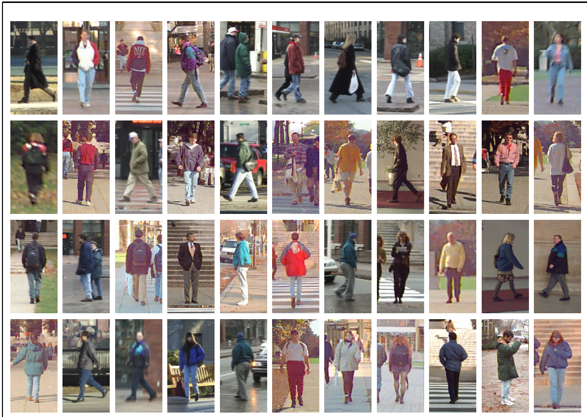
Figure 2-3: Examples from the database of people used for training. The images are color of size 128 \times 64 pixels. The examples vary in pose, color, texture, and background.
