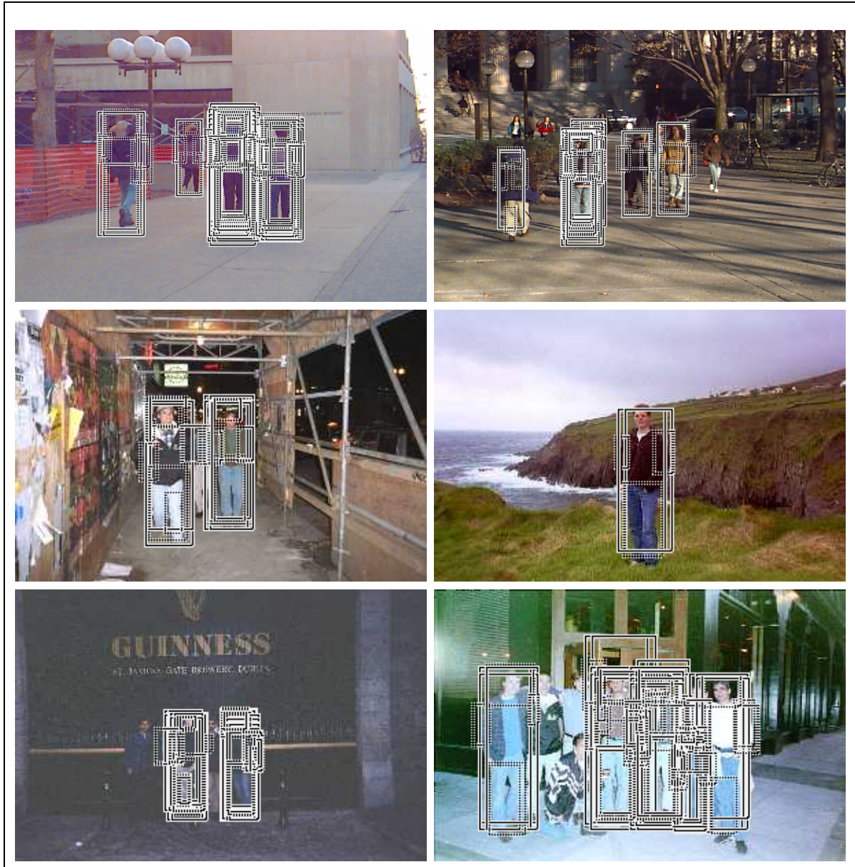
Figure 4-9: Results from the component based person detection system. The solid boxes outline the complete pedestrian, where the dashed rectangles are the components.
