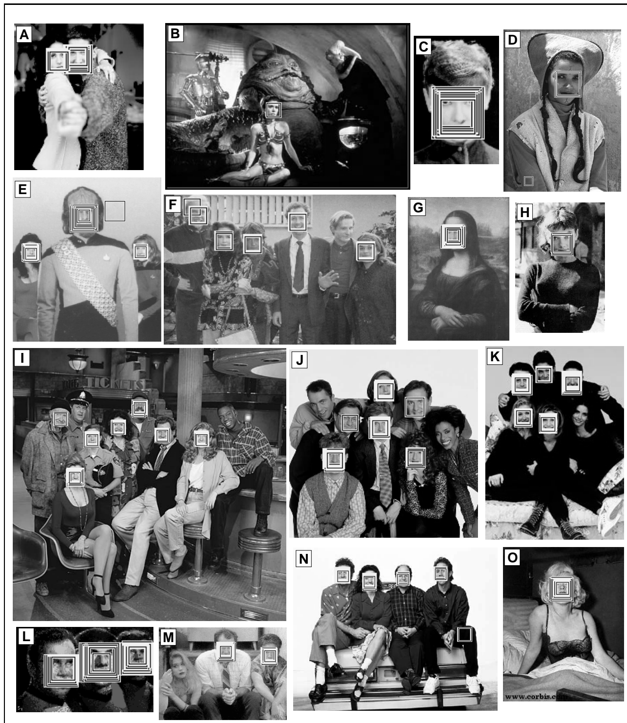
Figure 2-13: Results of our face detection system on a set of out-of-sample images. A, C, E, F, G, H, I, J, K, L, M, N are from the test database of Sung and Poggio; B, D are from www.starwars.com ; O is from www.corbis.com . Missed faces (B, F, I, J, K, M) are due to significant head rotations that were not present in the training data. False positives (E, F, N) are due to insufficient training data and can be eliminated by using more negative training data. The face detection system processes approximately 125,000 patterns per image.
