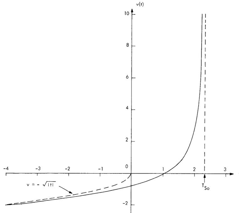
Fig. XVI-1. Solution of the dimensionless switching equation (3) with  $n(t) = 0$ . Initial condition was  $v_0 = -\sqrt{|t_0|}$  for  $t_0 \ll 0$ . The switching time  $T_{SO}$  is shown.
