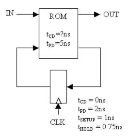
A. If the register is N bits wide, what is the appropriate size of the ROM? Give the number of locations and the number of bits in each location.
