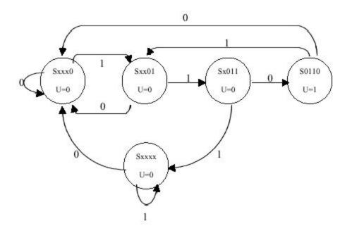
The name of each state represents how many digits in the sequence have been input. State Sxxxx indicates that the sequences has not begun, Sxxx0 indicates that the first 0 has been input, etc.
