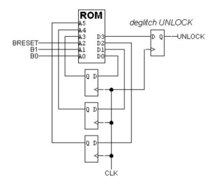
The button circuitry converts each button press into a single pulse guaranteed to be stable the required amount of time before and after the rising edge of the clock. For example, pressing "B0" once produces the following waveform:
