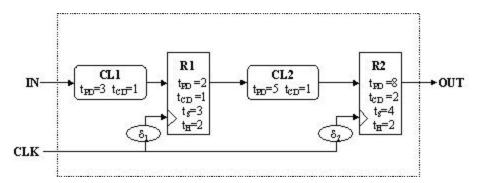
D. Rewrite the timing specifications for the system as a whole taking into account d1 and d2. Don't make any assumption about the relative sizes of the two delays.
