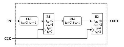
The components labeled CL1 and CL2 are combinational; R1 and R2 are edge-triggered flip flops. Timing parameters for each component are as noted.
