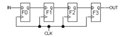
Each of the edge-triggered D flip-flops has a setup time of tS, a hold time of tH, a propagation delay of tPD and a contamination delay of tCD. Assume that IN is stable tS before the rising edge of CLK and tH after the rising edge of CLK.
