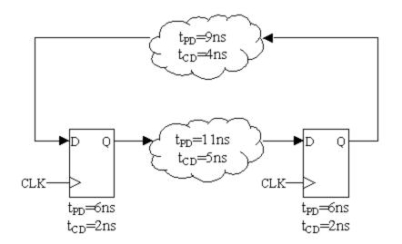
A. Assuming that the clock period is 25ns, what is the maximum setup time for the flipflops for which this circuit will operate correctly?
