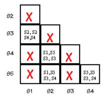
C. Finally, look at an entry (SI,SJ). If entry is "SM,SN" and if (SM,SN) has an "X", put an "X" in square (SI,SJ). Repeat until no more squares can be X'ed out. The remaining squares indicate equivalent states. Show the final state (no pun intended) of your compatibility table.
