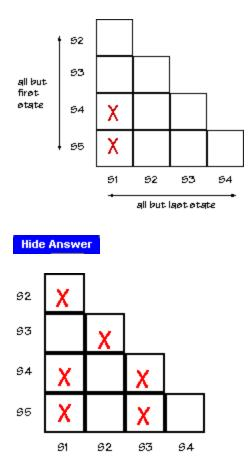
B. For each non-X square (SI,SJ) write in pairs of states that have to be equivalent in order for SI and SJ to be equivalent. For example, for S2 to be equivalent to S5, then S1 (where S2 goes with a "0" input) has to be equivalent to S5 (where S5 goes with a "0" input).
