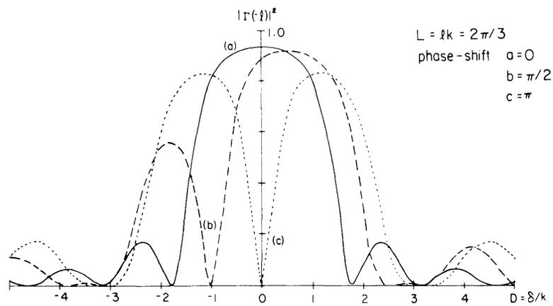
Fig. VIII-1. Reflection spectra for a waveguide with three different phase shifts.  $D = (\beta - \beta_0)/\kappa$ .
