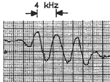
Figure 22.5 Ramsey fringes for a 7.5 cm zone separation.
