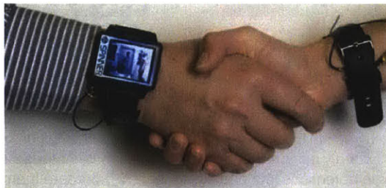
9 Early prototype of the SPINNER wrist sensor unit provides gesture data and galvanic skin response
