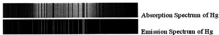
Figure 2-2: A representation of the absorption and emission spectrum of Mercury. The resonance condition implies that the absorption spectrum is the photonegative of the emission spectrum [41].
