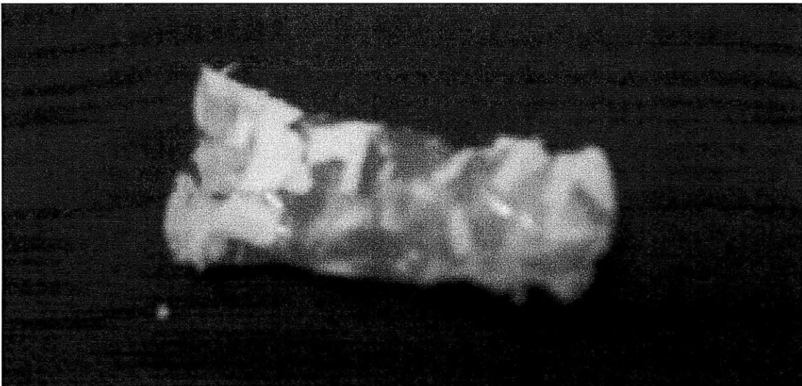
Figure 3.17: Paint flaking off of a painted balloon
