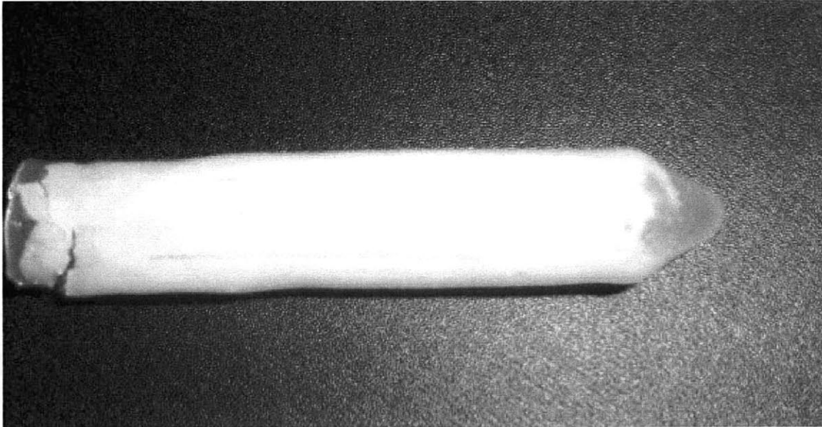
Figure 3.18: Balloon made with layer of fluorescent paint trapped between two layers of urethane
