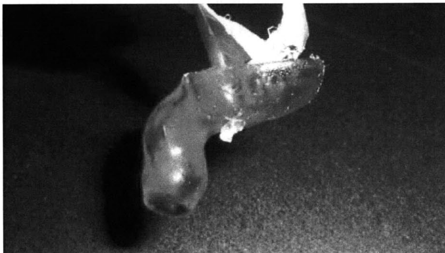
Figure 3.7: Hard plastic hearing aid shell to be used for mold as balloon.
