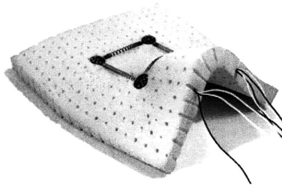
**Figure 1:** *Surflex* is a tangible SMA device as well as a platform for sensory feedback experimentation. Developed by Marcelo Coelho at the MIT Media Lab
