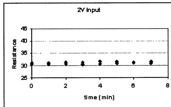
**Figure 6:** A 2 Volt drop was maintained over the test setup. Resistance of the spring oscillates slightly over time.
