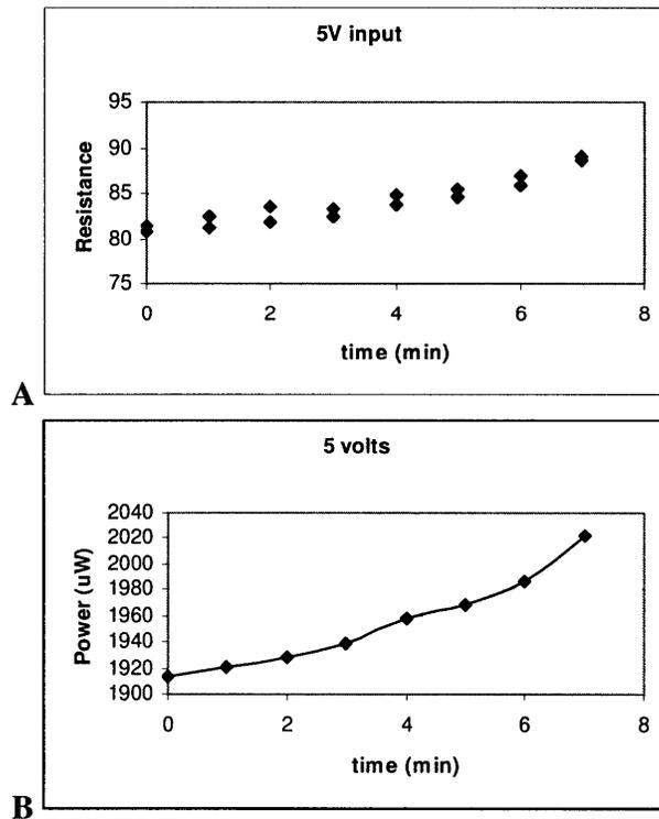
**Figure 7:** A 5 Volt drop was maintained over the test setup. A) The resistance drifts upwards over time. B) The power input to the spring increases with time due to the increase in resistance
