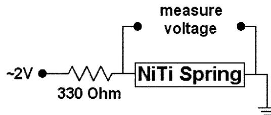
**Figure 5:** A voltage divider circuit is used to determine the resistance of the Nickel-Titanium spring. The voltage drop across the test setup remains constant at 2 Volts
