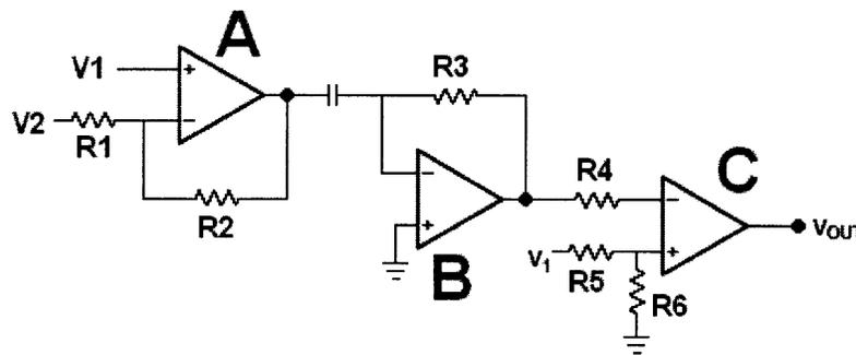
**Figure 13:** The output of this circuit is a digital signal which represents the strain rate of the spring sensor. A) Differential amplifier receives inputs from Wheatstone Bridge. B) Differentiator. C) Comparator.
