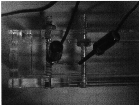
**Figure 4:** An acrylic test jig was designed to control and measure the displacement of the superelastic springs
