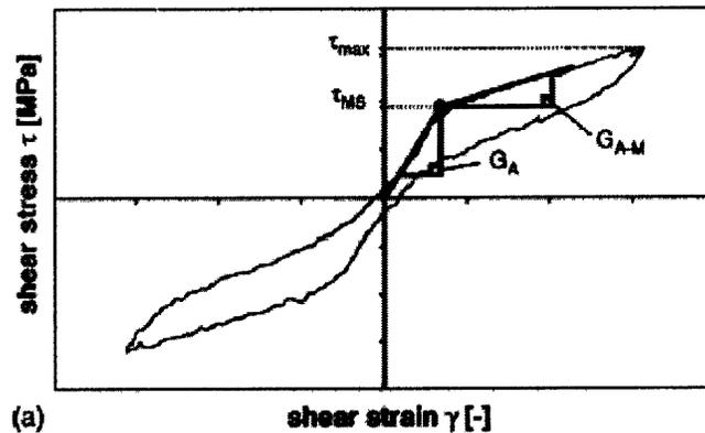
**Figure 11:** Stress-Strain behavior of Nickel-Titanium from Predki, et al.
