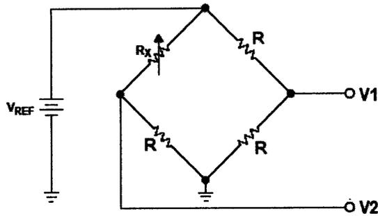
**Figure 12:** The Wheatstone Bridge is commonly used for precision resistive sensing.  $R_x$  represents the sensor.
