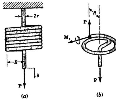
**Figure 2:** The coil spring converts small torsional motion of the wire into large axial displacements. Diagram from *An Introduction to the Mechanics of Solids* by Crandall.
