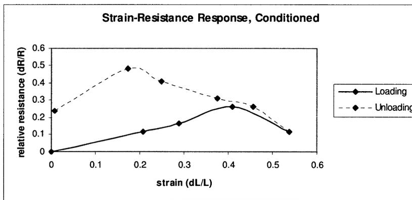
**Figure 10:** A 2 Volt drop was maintained over the test setup. The strain-resistance response is nearly linear up to 40% strain. The behavior is highly hysteretic.
