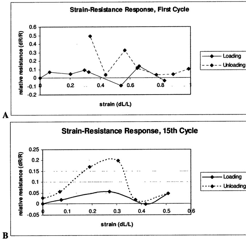
**Figure 9:** A 2 Volt drop was maintained over the test setup. A)The resistive response of a freshly made spring was very irregular. B)After being deformed 15 times, the strain-resistance response stabilizes
