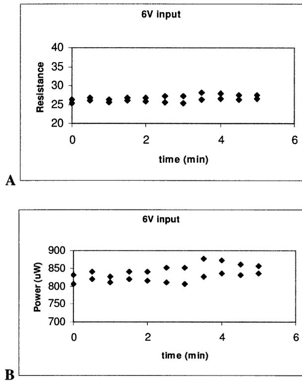
**Figure 8:** A 6 Volt drop was maintained over the test setup. A)The resistance enters a hysteric loop which stabilizes the effect of Ohmic heating. B)The power input to the spring fluctuates over time.
