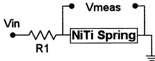
**Figure 3:** A voltage divider circuit is used to determine the resistance of the Nickel-Titanium spring
