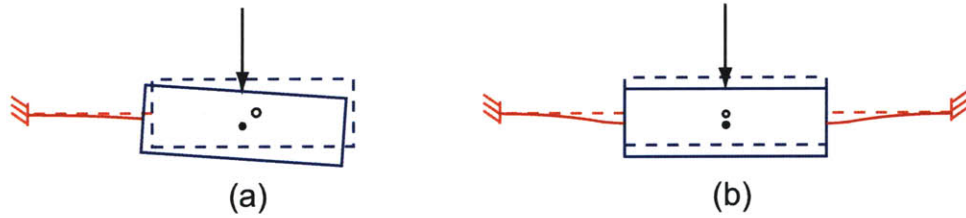
Figure 5-10: Primitive beam flexure shown in (a) is enhanced in its load-capacity by adding a redundant constraint in (b) to produce a double-sided beam flexure primitive.
