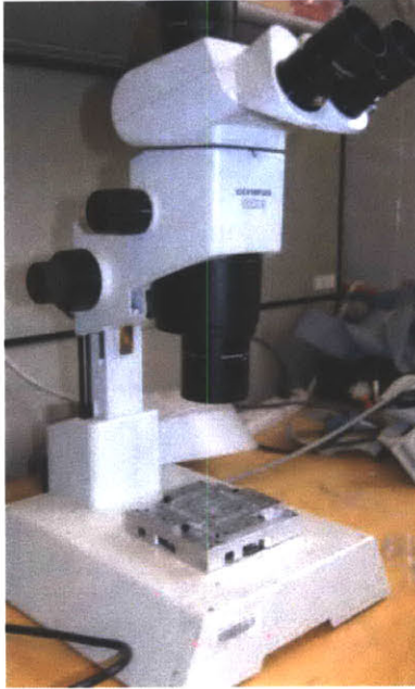
Figure 6-13: Optical registration against crosswires of a microscope allows for XY alignment of the Z rod flexures before they are bonded to the central stage.
