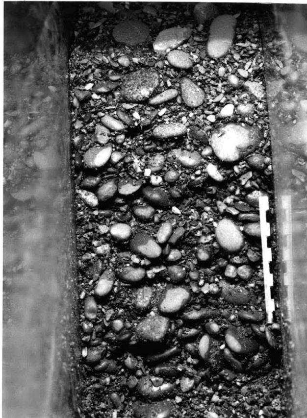
Figure 5-20 : Deposit of Run 5: Flow-parallel and Flow-normal Cross-sectional Views
