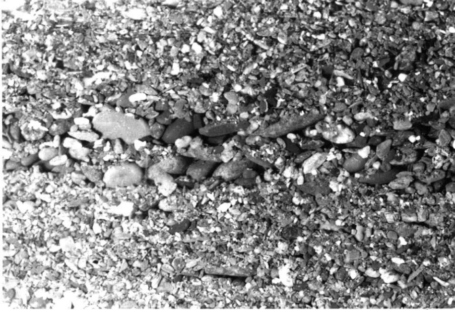
Figure 5-21 : Openwork Gravel Lenses Formed During Run 5
