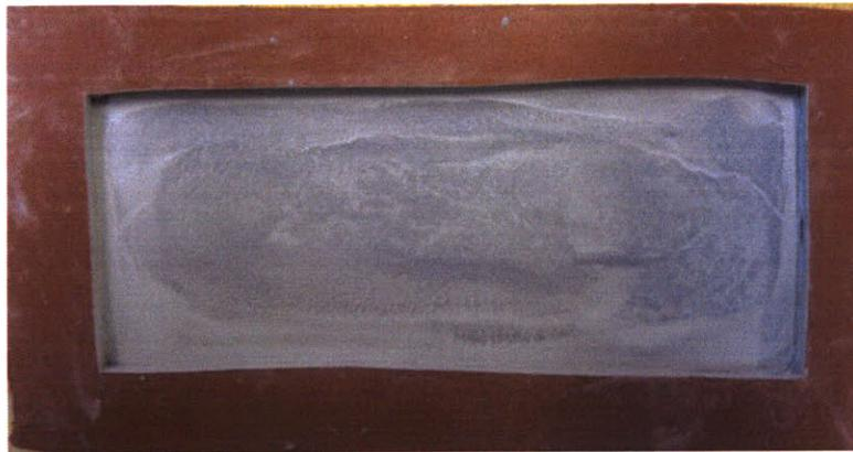
**Figure A1:** Photograph of powder slurry cast on top of the wafer and backing plate. The orange frame is a 1 cm thick piece of silicone rubber used as a mold to contain the slurry as it is poured over the wafer and backing plate. The grayish middle rectangle is the powder slurry after it has been allowed to set in air. The rubber mold is subsequently removed and the powder is sintered in a box furnace.
