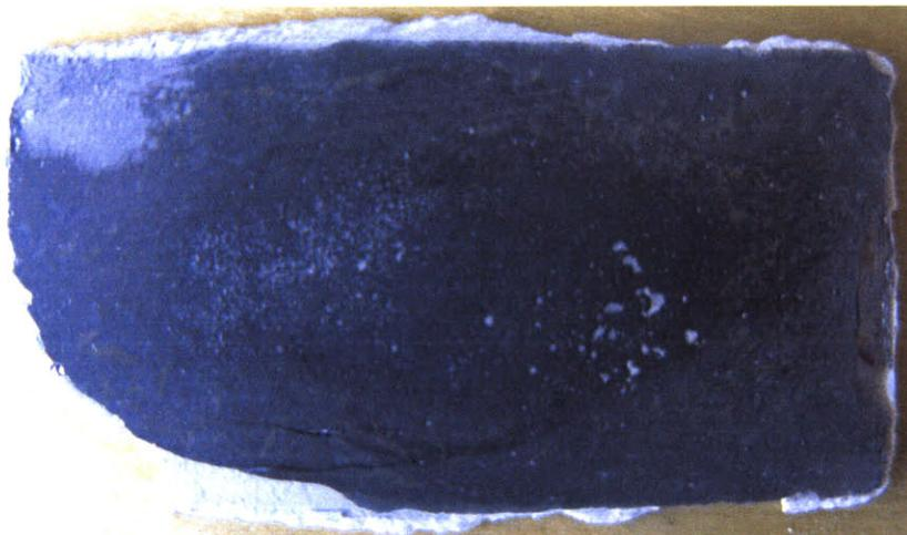
**Figure A13:** Photograph of the underside of a wafer that was recrystallized with a SiC/alumina bimodal powder shell. The resultant wafer has a scalloped texture. The test implies that a completely rigid powder shell is needed to contain a wafer during recrystallization.
