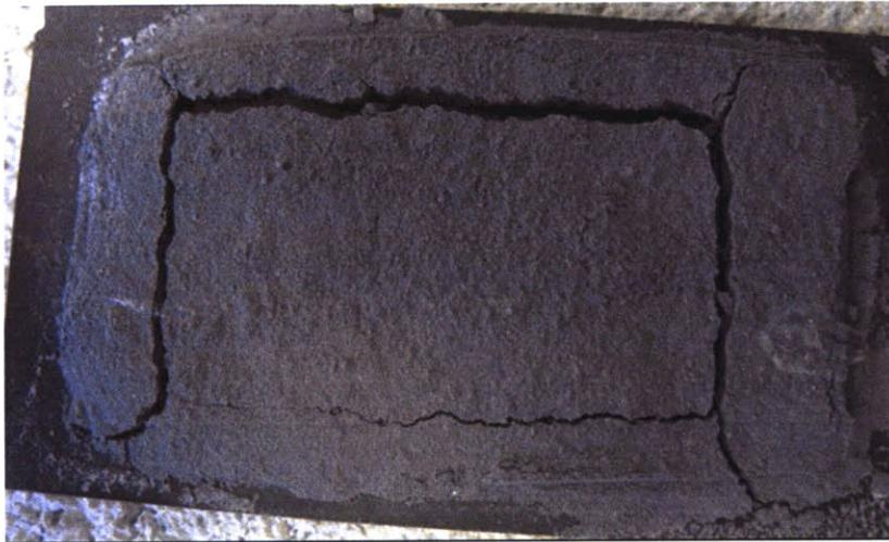
**Figure 40:** Photograph of powder shell following recrystallization. SiC bimodal powder completely surrounded the wafer. With powder on both sides of the wafer, the shell developed large cracks, leaving us unable to create an intact enclosure.
