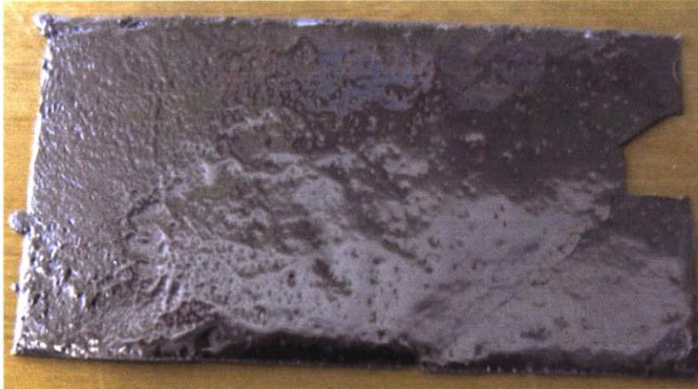
**Figure 27:** Photograph of the bottom surface of a wafer following recrystallization within a SiC powder shell. The left edge of the wafer is the leading edge. The wafer has a very rough surface finish with frequent pits due to powder particles in contact with the wafer itself.
