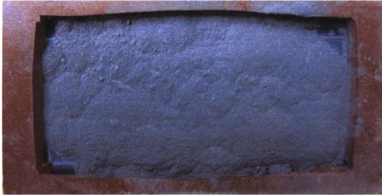
**Figure 25:** Photograph of the recrystallization setup after powder has been poured over the wafer and vibrationally compacted. The rubber mold keeps the powder from spilling off of the backing plate. The powder bed is not a perfect layer, but is an improvement over the initial state of it after is been poured onto the wafer.
