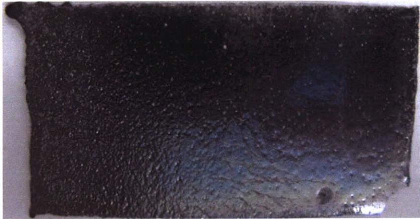
**Figure 8:** Photograph of a wafer recrystallized with parallel backing plates. The right side of the photograph is the leading edge and the left side is the trailing edge. The non-uniformity on the trailing edge of the wafer displays how poorly parallel backing plates preserve the geometry of a wafer during recrystallization.
