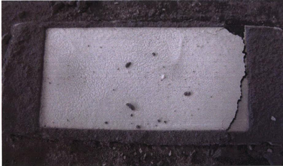
**Figure 42:** Photograph of cast silica release layer after recrystallization has occurred. The wafer was easily removed from the release layer which remained flat and intact during the melting process. The layer also sintered slightly, creating a layer which would support the molten wafer.
