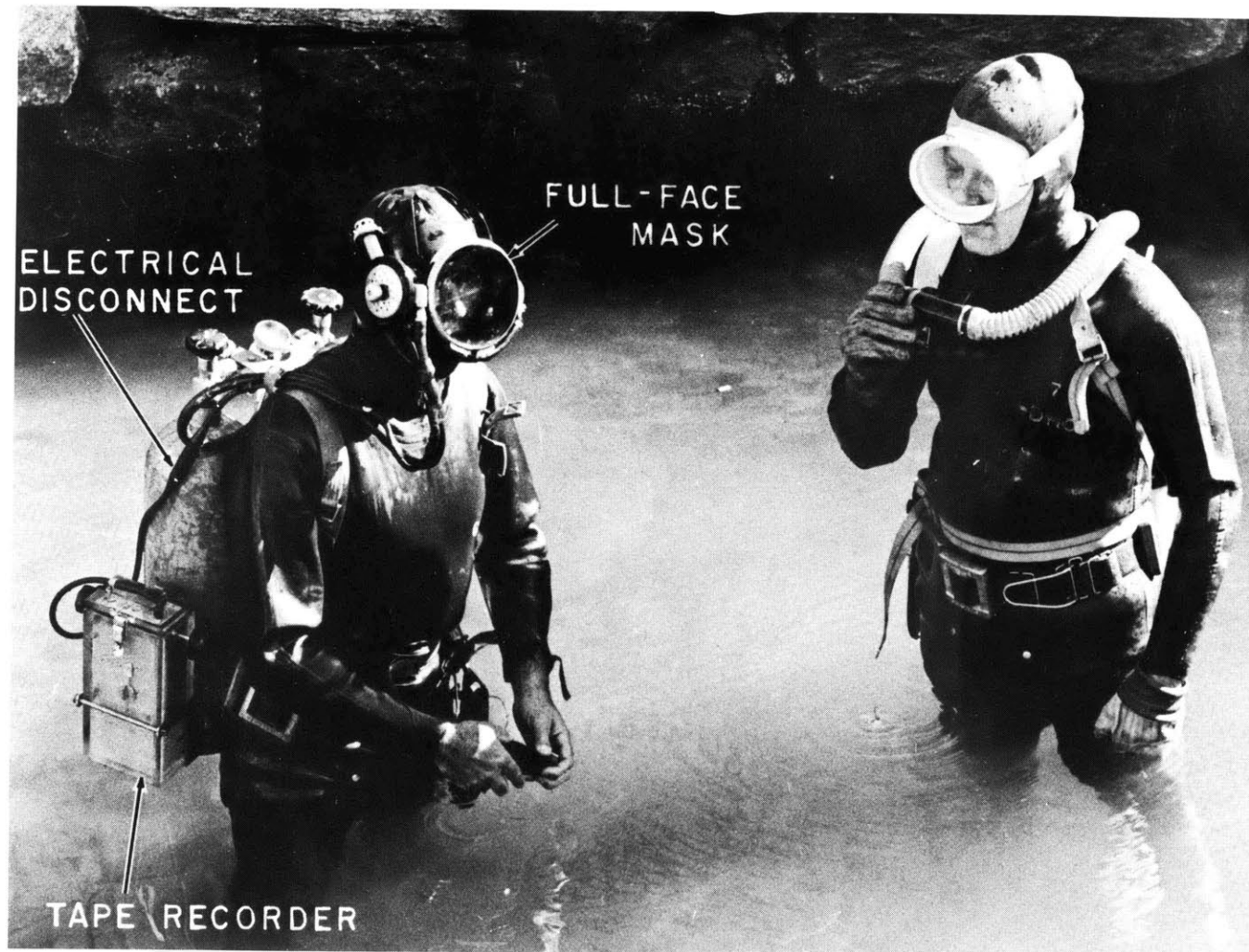
Figure 19. Photograph of the Self-Contained Portable Tape Recording System being Worn by a SCUBA Diver.
