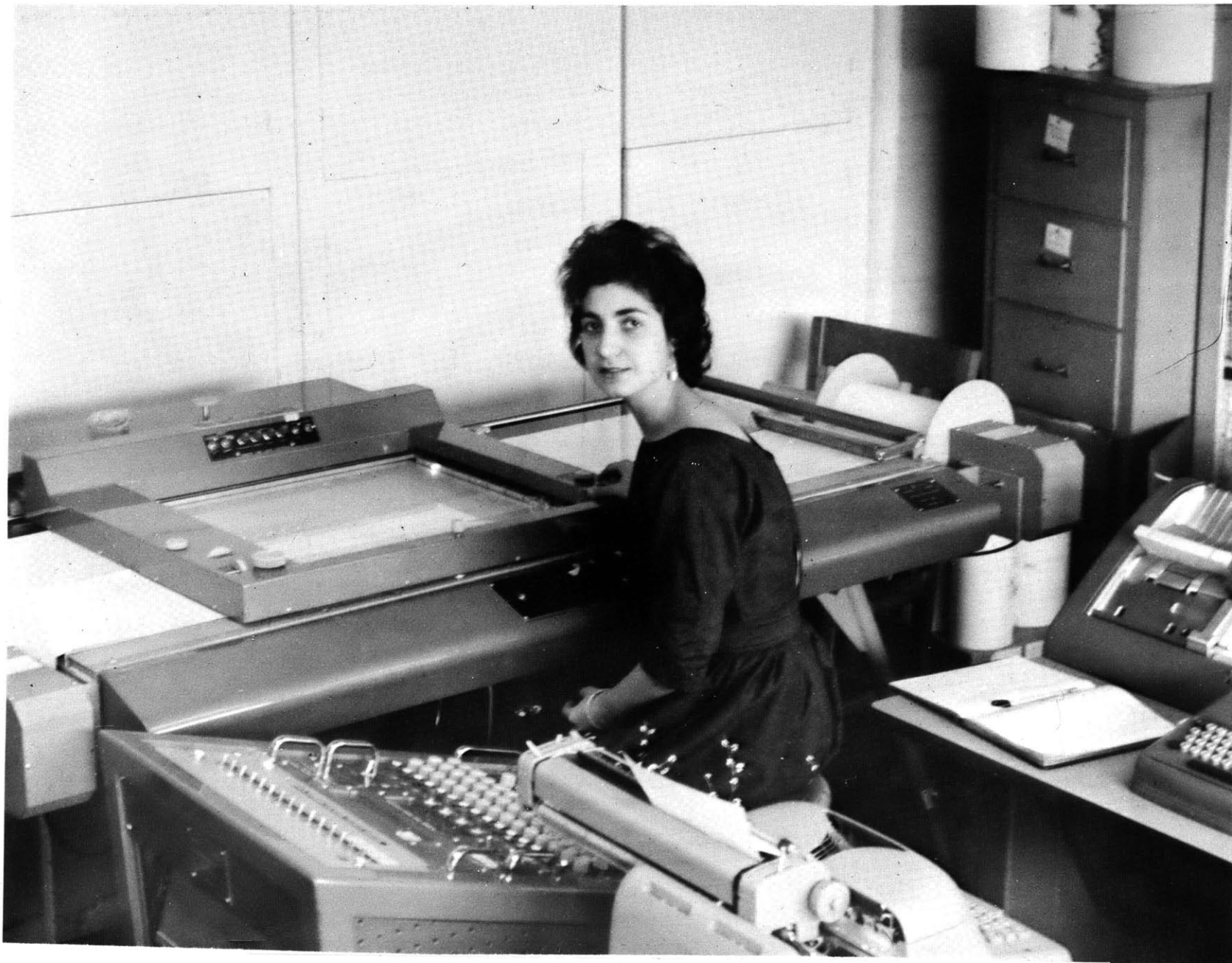
Figure 22. Photograph of the Analogue to Digital Data Reduction System being used to Digitize the Acoustic Echoes.
