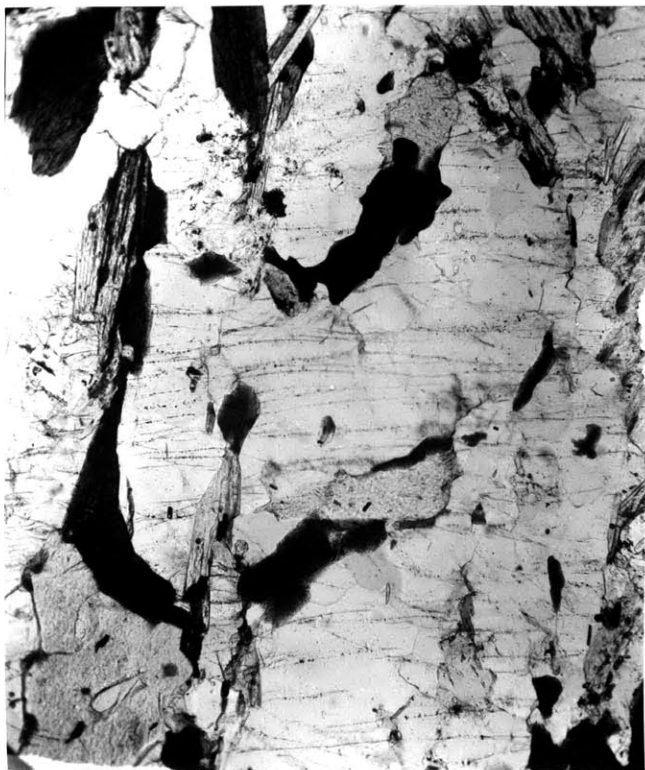
Figure 7. Photomicrograph of thin-section of gneiss showing planes of liquid inclusions as lines or rows of dark specks in quartz grains. x 30.
