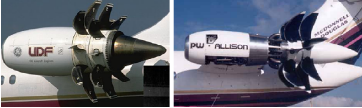
Figure 1-1: GE UDF flight test on MD-80 in 1988 (left) and PW/HS/Allison 578-DX flight test on MD-80 in 1989 (right)
