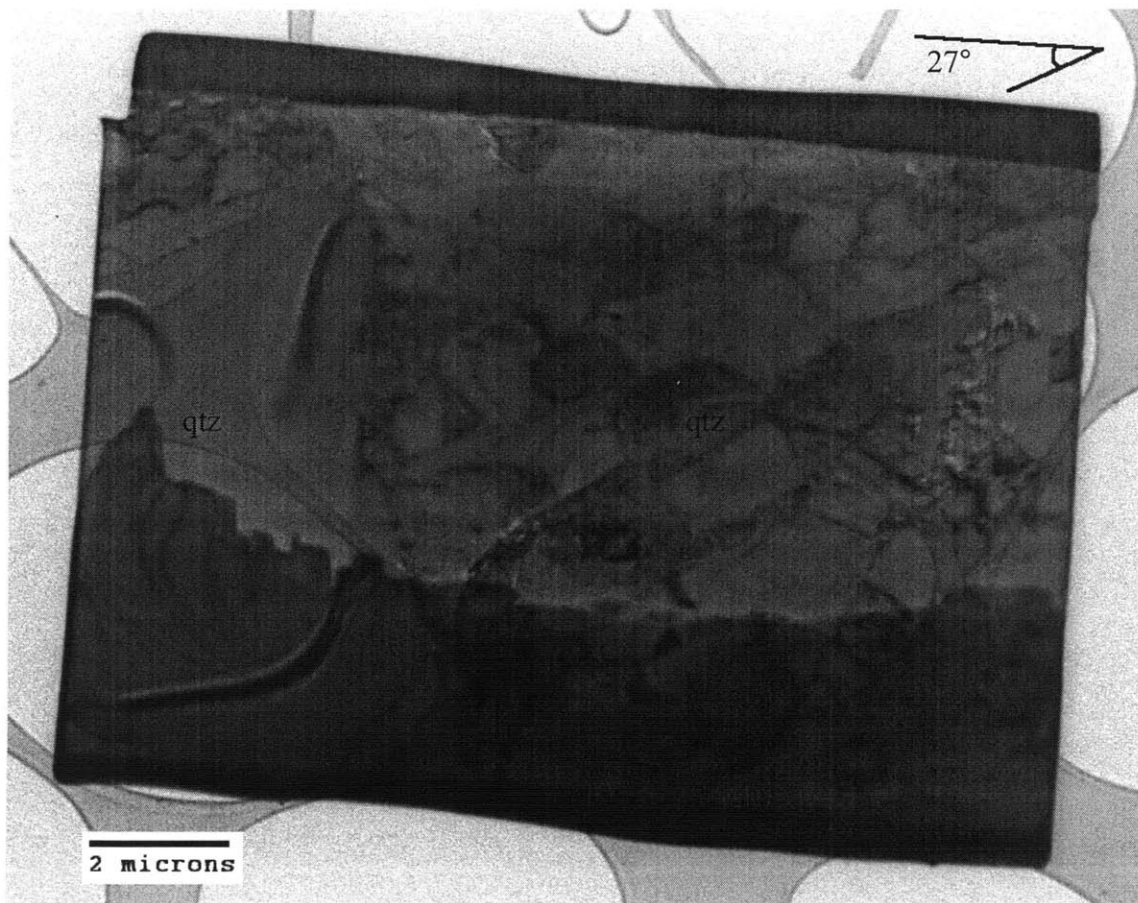
Figure 6. Sample 635 was deformed at 973 K to a total shear strain of 3.27 under a differential stress of 96 MPa. The wedge at the top right shows the angle between the direction of shearing (parallel to the top sample edge) and the major axis of the finite strain ellipse. The clear region at the left of the sample is a large quartz grain, as is the small clear grain near the center of the sample (both labelled “qtz”). The darkening present in the lower third of the sample is caused by the sample being thicker in that area from fracturing during sample preparation. The background is a holey carbon film.
