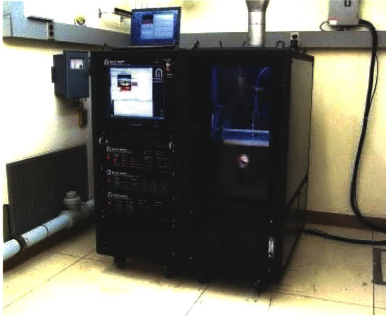
Figure 2-4: The commercially available Black Magic CNT deposition system produced by Nanoinstruments, Ltd. located inside the MTL.
