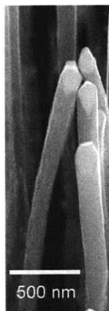
Figure 4-28: A CNT possibly bent due to magnetic attraction force from adjacent CNT.
