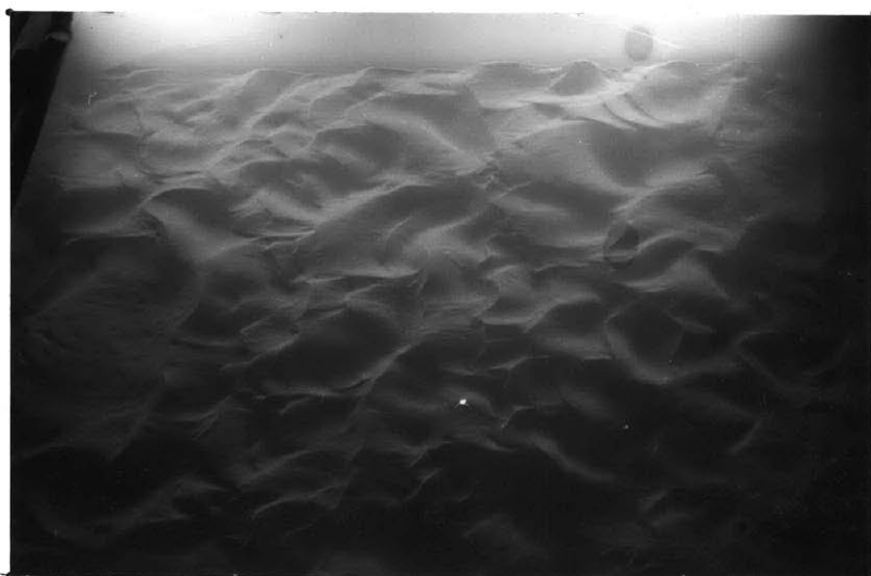
Fig. 4.7. Run IV-26, U = 58 cm/sec. Bars plus ripples. Outline of bar to far left; side of bar shaded in fore- ground. Note flat trough.
