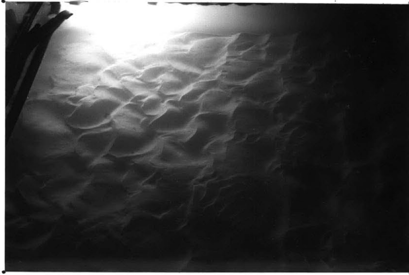
Fig. 4.8. Run IV-25, U = 60 cm/sec. Bars plus ripples. Bar to right, with continuous crest and flat relatively long trough.
