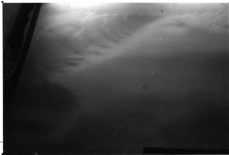
Fig. 4.15. Run IV-15, U = 84 cm/sec. Dunes. Cusped, rippled dune front (upper left). Streaks normal to slip face (lower left). Transitional between dunes and flattened dunes.
