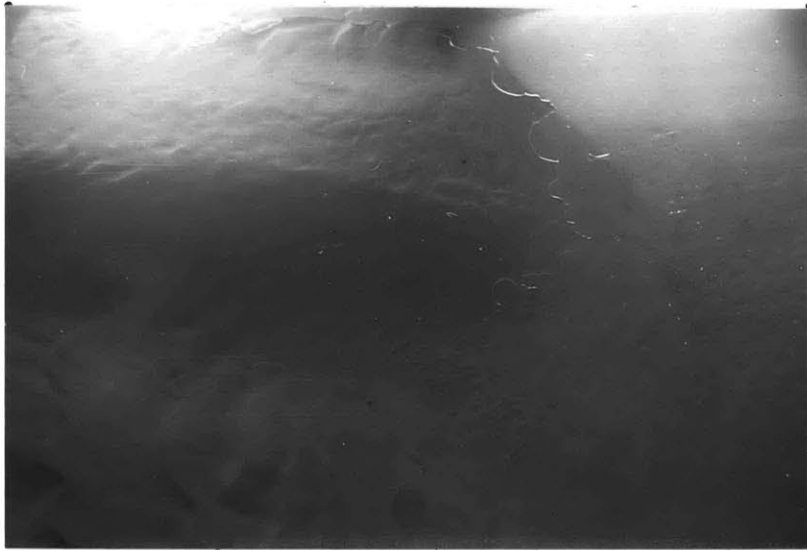
Fig. 4.14. Run IV-13, U = 84 cm/sec. Dunes. High, straight-crested, flat-backed dune. Well-defined trough with en echelon ripples. Note streaks normal to crest. Lineations at base of slip face indicative of cross-currents in trough.
