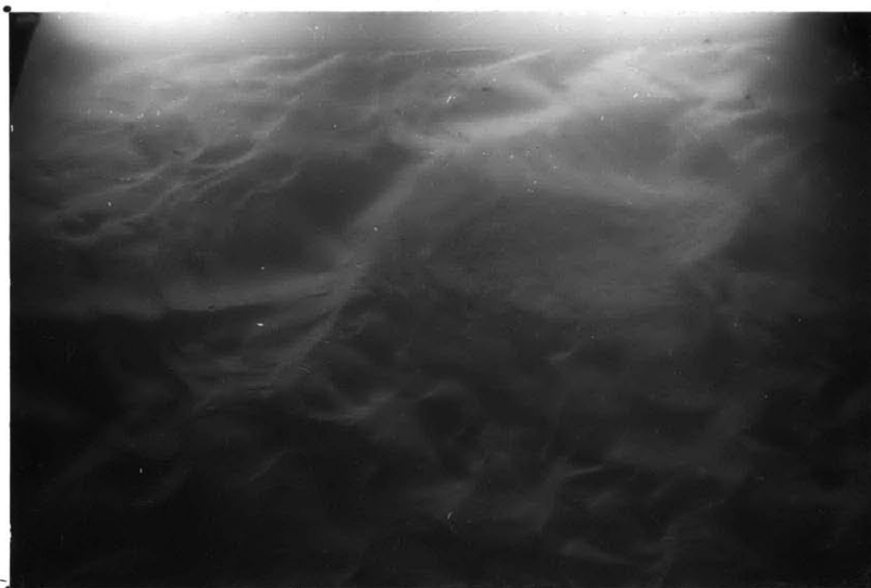
Fig. 4.11. Run IV-22, U = 67 cm/sec. Bars plus dunes. Semi-continuous crests. Flattish bar trough to right; scoured dune trough to left.
