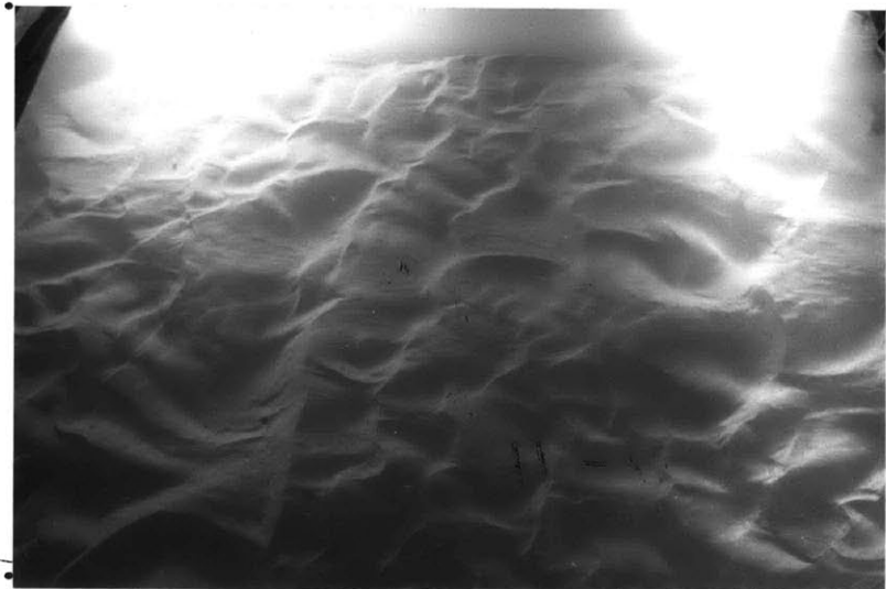
Fig. 4.9. Run IV-24, U = 64 cm/sec. Bars plus ripples. Bar with continuous crest, higher than ripples.
