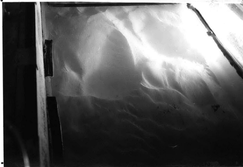
Fig. 4.12. Run IV-8, U = 72 cm/sec. Dunes plus ripples. Scoured, unrippled trough and rippled dune-back. Flow from bottom to top.
