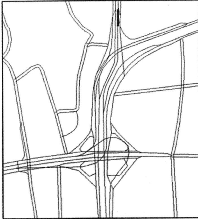
Figure 3-9: A Typical Freeway Short Link #372
