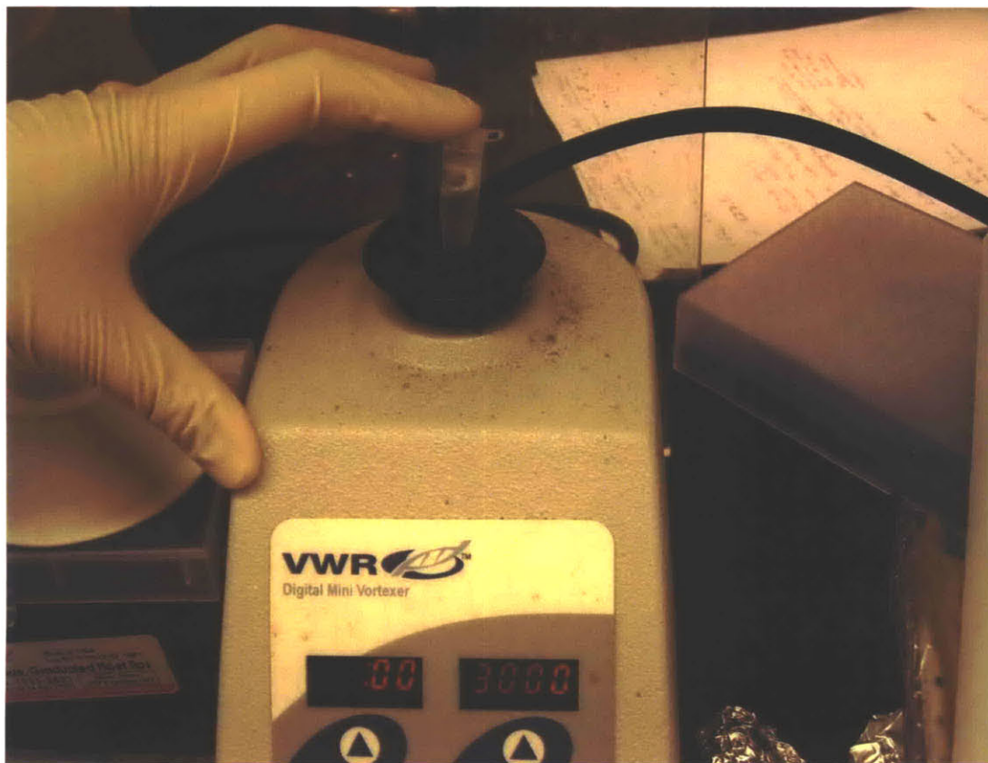
Figure C.1 Vortex the sample using a bench top vortex machine for 30 seconds to fully disperse the fatty acid in the NaOH solution.
