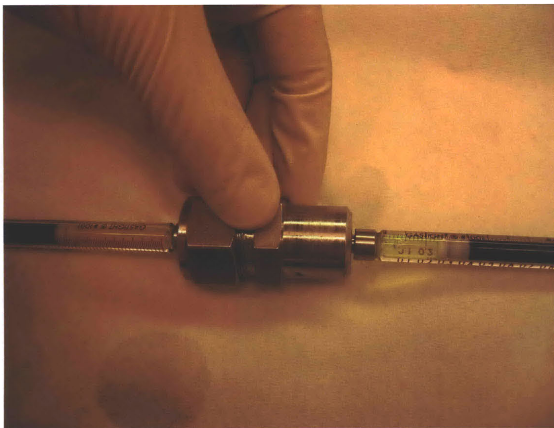
Figure B.4 Slowly push one syringe (left), so that all the solution in it goes through the hand-held mini-extruder to the other side, into the other syringe (right).
