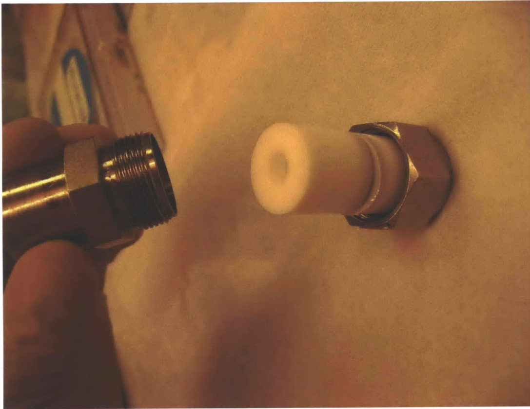
Figure B.3 Assembly of the internal membrane support parts with filter support and polycarbonate track-etched membrane in the middle.
