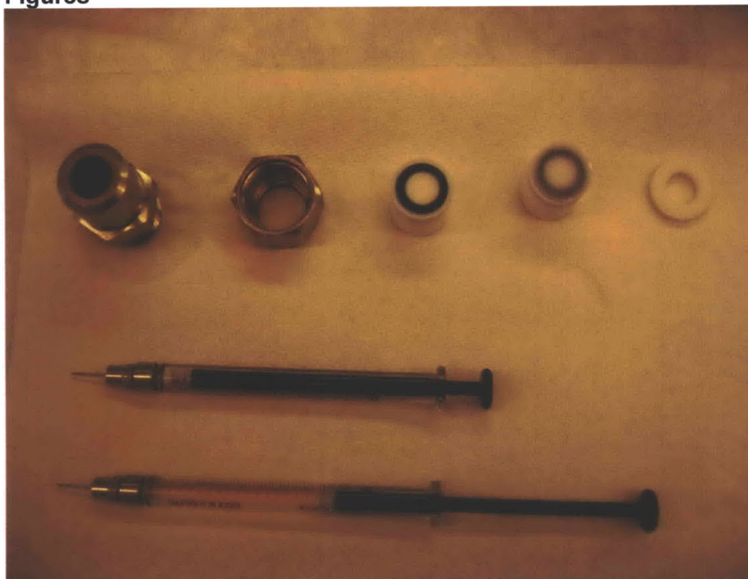
Figure B.1 Hand-held mini-extruder with two gas-tight syringes.
