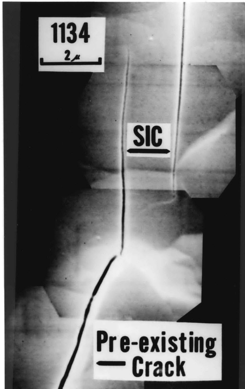
Figure 3-8. Stress induced elongation of pre-existing crack in quartz. SIC are parallel to the direction of maximum compression. SEM micrograph of sample 1134-9.
