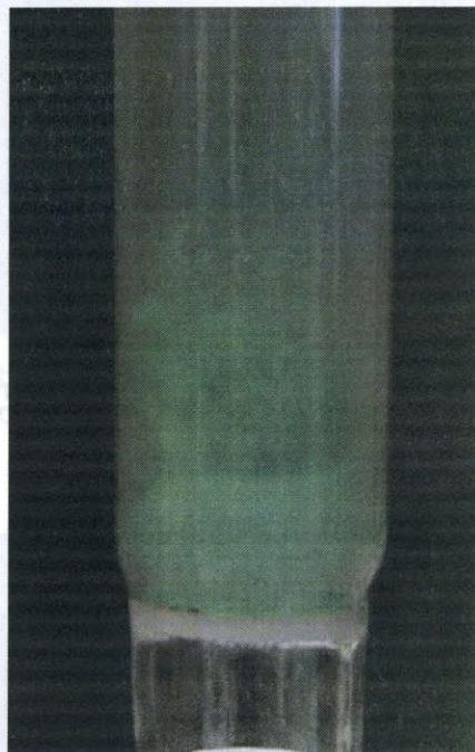
Figure 3.4 – Detail of Full Scale Glass Column During Operation : Fluidization is evident from the appearance of the bed.
