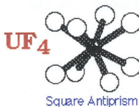
Figure 2.2 – Structure of Uranium Tetrafluoride
