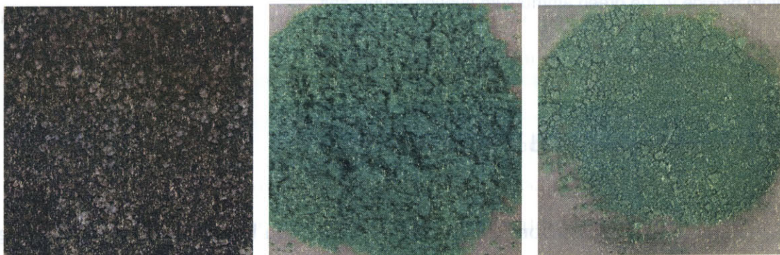
Figure 5.3 – Ambient Temperature Fluorination, Fine \text{UO}_2 : When the brown reagents (left) were ground in a ball mill for twenty minutes, a pronounced color change to bright green (center) occurred. After the powder was fluidized in argon for two days, the color was slightly lighter (right).
