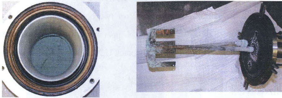
Figure 3.1 – Stirred Bed Apparatus: A crucible sat within the reactor vessel (left) and reactants were stirred by a paddle (right). The coating of rust visible in these pictures was the result of corrosion of mild steel shimstock that had been attached to the paddle to aid in complete mixing. Very little corrosion of stainless steel parts was seen.
