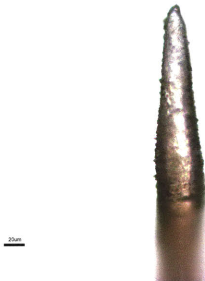
Figure 6 | PLGA microneedle at 20 \mu m point after removal from the first conical PDMS mold
