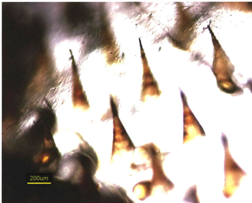
Figure 8 | PLGA with 0.10µm silica. The entire array consisted of repeating bands starting along the microneedles
