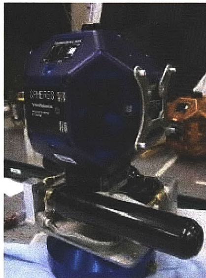
Figure 2-9. One of the SPHERES on the low-friction test bed at MIT.
