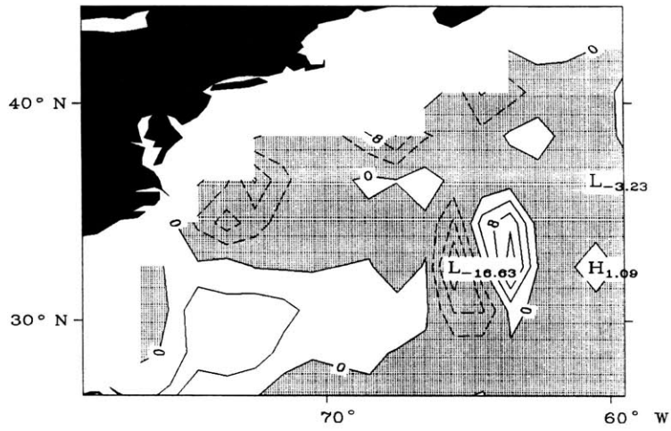
Figure 3.21: Two Terms in the Heat Budget: K_H T_{xz} - w T_z . (Scaled by 10^8 , interval 4)
