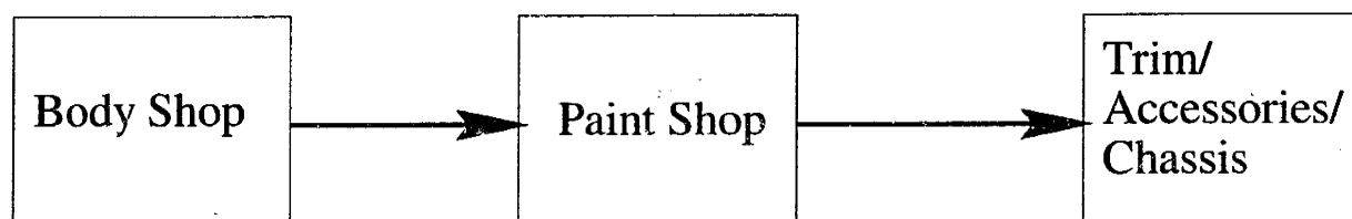
Figure 1-1: Stages of the automobile assembly process
