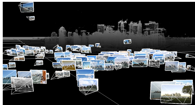
Fig 8. Approximately 500 reconstructed skyline photos georegistered with the 3D NYC map.
