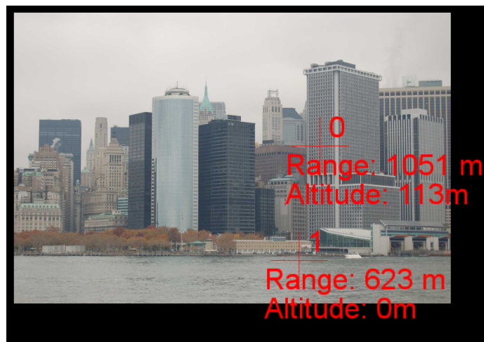
Fig 12. Points in fig 11b reprojected onto pixels in another photo. Camera ranges to features depend upon image, while urban feature altitudes remain invariant
