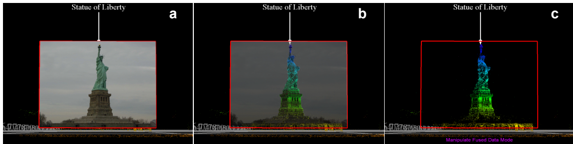
Fig 7. One Statue photo displayed in front of its reconstructed point cloud with (a) 0%, (b) 50% and (c) 100% alpha blending.
