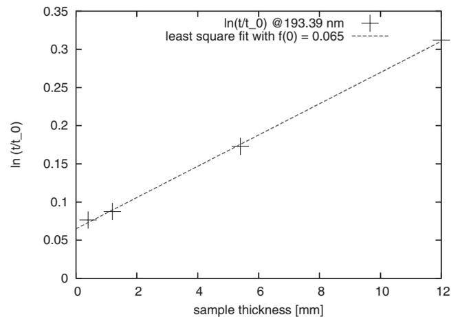
FIG. 7. The surface contribution for the wavelength of 193 nm can be extrapolated by plotting the quantity  $\ln(t/t_0)$  as a function of sample thickness. The y-axis intercept is the (dimensionless) surface absorption. For 139.39 nm, this is in our case 0.065 (based on log e).
