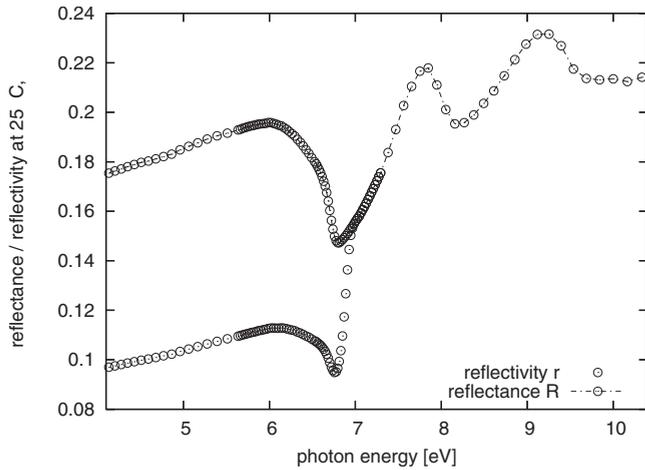
FIG. 4. The bare reflection  $r(\tau, R)$  (reflectivity), which accounts for multiple reflections, is plotted together with the (directly measured) reflectance  $R$  as a function of photon energy. For small photon energies there is a strong difference since the material is transparent and multiple reflections are important. For larger photon energies the material is in transparent, multiple reflection does not occur, and the two curves merge.
