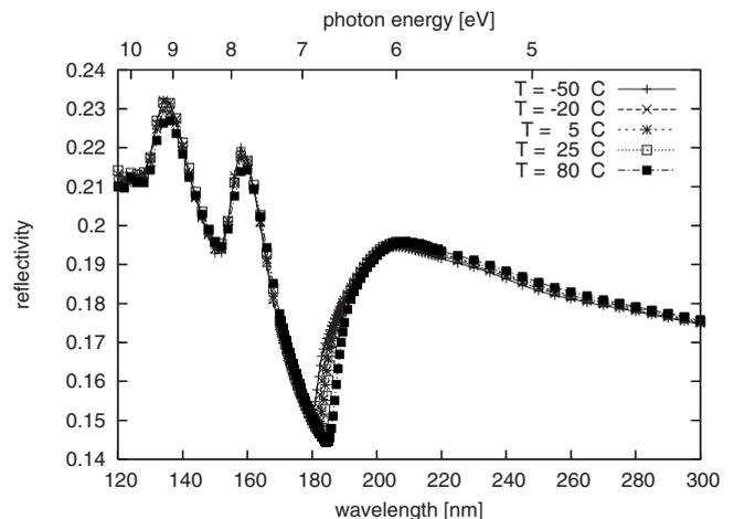
FIG. 3. Measured reflectance of the LuAG sample  $d=12$  mm, with the temperature as a parameter. The strong increase in the reflectance between 190 and 200 nm (6 and 6.7 eV) is due to the onset of transparency of the material, and the resulting (multiple) reflections from the rear surface.
