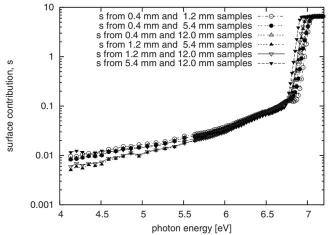
FIG. 6. The surface contribution  $s$  according to Eq. (8) plotted as a function of photon energy. The surface contribution obtained in this way is independent of the choice of the pair. This indicates a good and reliable surface polish.
