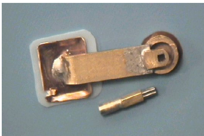
Figure 5 Mask holder and nozzle fixture: Left: Mask/nozzle holder and wrist fixture; Right: Close up of 4-hole mask and nozzles.
