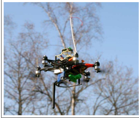
Fig. 1. Our six-rotor helicopter with bird's-eye video camera. The helicopter is 28cm in diameter and weighs 142g without the navigation electronics, camera or communication hardware.
