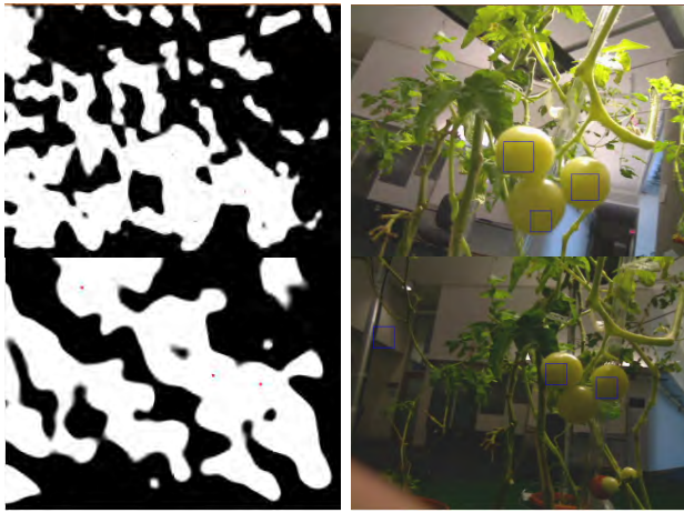
Fig. 4. Left : Result of convolution of input image with 40 feature/location pairs. Red dots correspond to local maxima. Right column : Detected fruits are highlighted with a rectangle. Notice the false-positive and misses in the bottom row.
